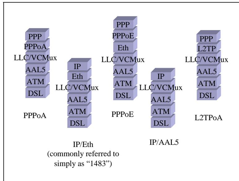
Figure 3: Protocol Stacks at the "U" Interface
