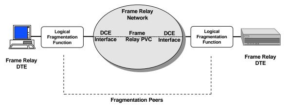
Figure 4-3 End-to-End Fragmentation/Reassembly Reference Diagram
