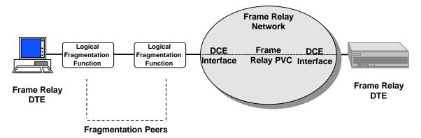
Figure 4-1 UNI Fragmentation/Reassembly Reference Diagram
