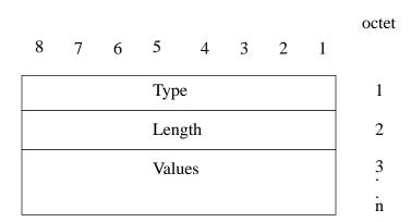
**Figure 7 - DCFD Configuration Option Format**
