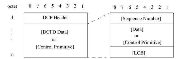
Figure A.1 - Format of DCP PDU
