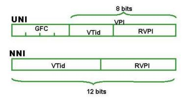
Figure 9 Bit-aligned VTs
