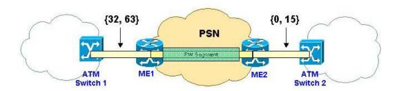
Figure 10 Reconciling differently-sized VPI ranges
