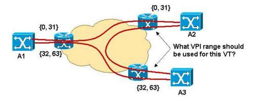
Figure 6 Example of the problem that arises when VPI Ranges cannot be modified by MEs
