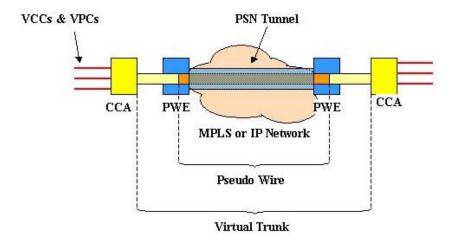
Figure 1: Generic Virtual Trunk Architecture
