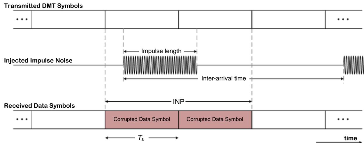
**Figure 5: Reference signals demonstrating impact of impulse noise.**
