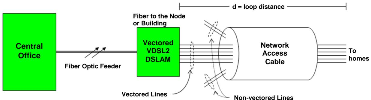
**Figure 3: Reference Fiber Fed DSL Network Access Architecture.**
