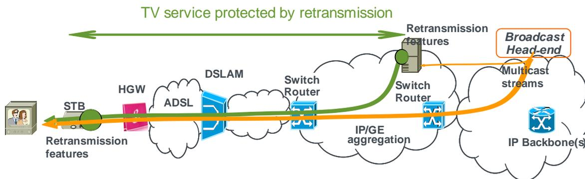
**Figure 6: Network architecture for retransmission**
