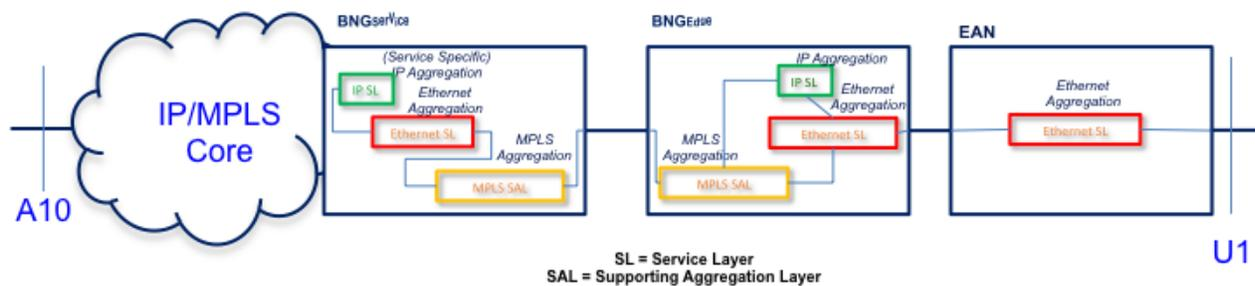
**Figure 3 : BNG Hierarchies, High Level Functional Distribution**
