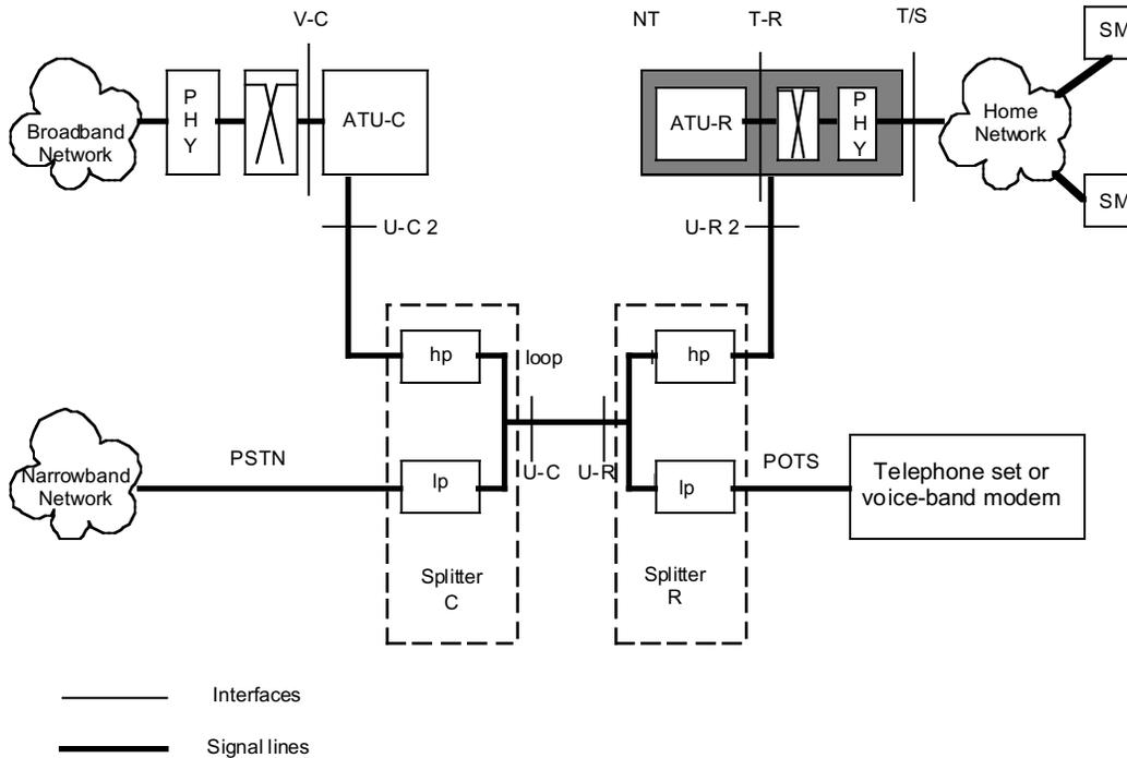
**Figure 1 ADSL Forum System Reference Model**
