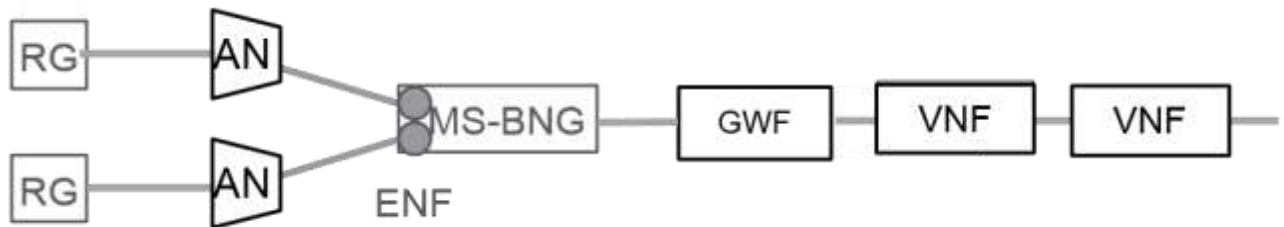
Figure 11 – ENF Model 2: ENF is hosted on an MS-BNG
