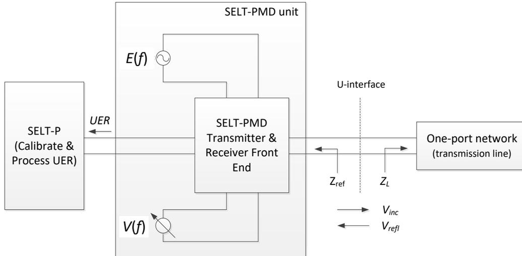
Figure 1: SELT Reference Model for calibrating CPE SELT
