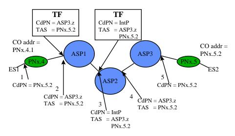
Figure 1.4- 2 Multi Level Address Stack Example
