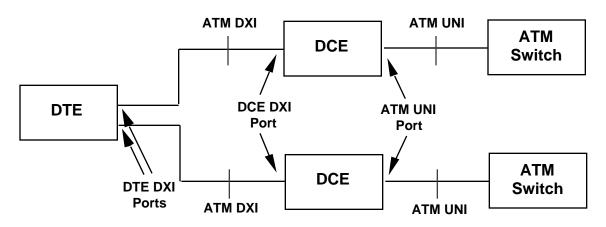
Figure 4.2 DTE/DCE Configuration for the ATM DXI LMI
