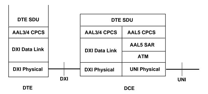
Figure 2.10 Mode 2 Protocol Architecture for AAL5
