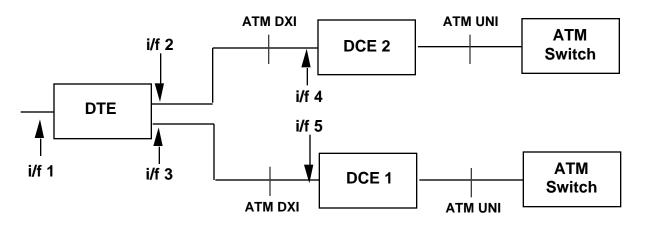
Figure 4.3 Example of Interface Indices for MIB-Centric Approach
