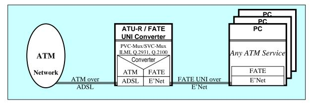
Fig 4.2. Multi-PC support with Intelligent ATU-R
