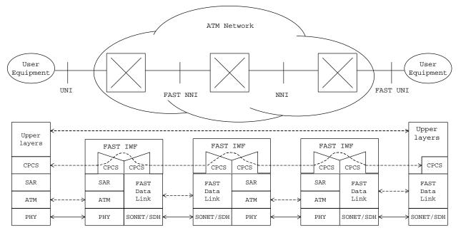
Figure 3 - FAST IWF Deployment Options
