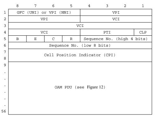
Figure 14 - OAM PDU encapsulated in FAST mode 1 frame
