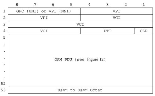
Figure 13 - OAM PDU encapsulated in FAST mode 0 frame
