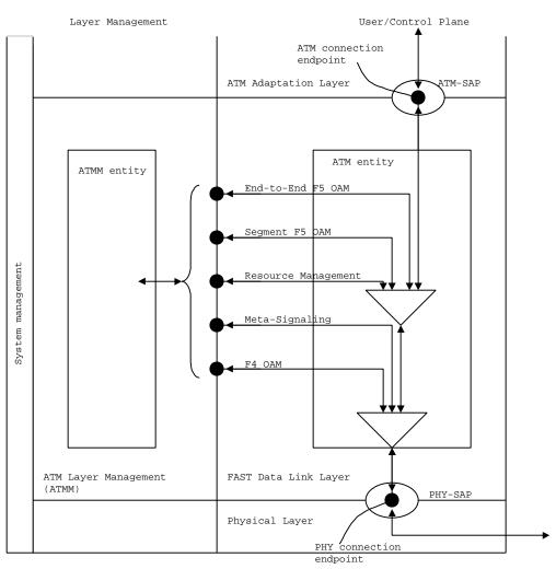
Figure 11 - Relationship of the ATMM and FAST Data Link Layers
