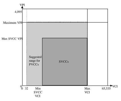
Figure 4 - Switched VCC VPI and VCI Values
