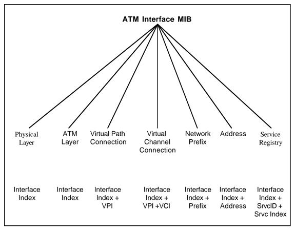
Figure 2 - ATM Interface MIB Tree Structure
