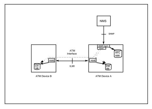
Figure 6 - NMS access to ILMI MIBs through Proxy-agent
