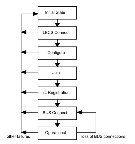
Figure 8. Initialization, Recovery and Terminating the ELAN
