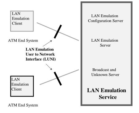
Figure 2. The LAN Emulation User to Network Interface (LUNI)
