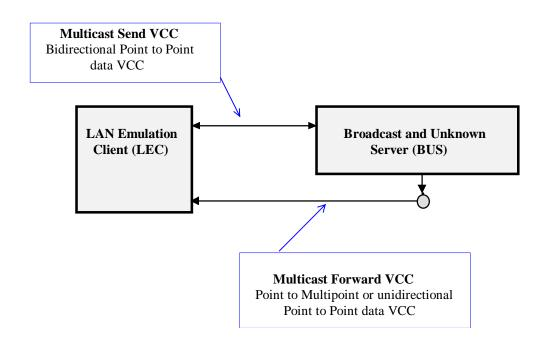
**Figure 7. LAN Emulation Client to BUS Connections**
