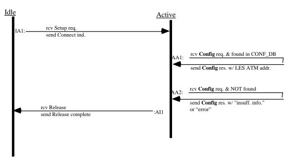
**Figure 15. LE Configuration Server State Machine**
