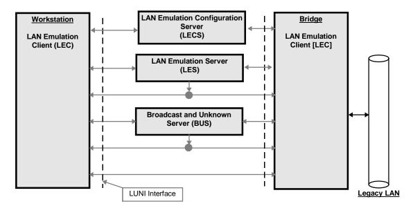
Figure 3. Basic LAN Emulation Client Connections across LUNI
