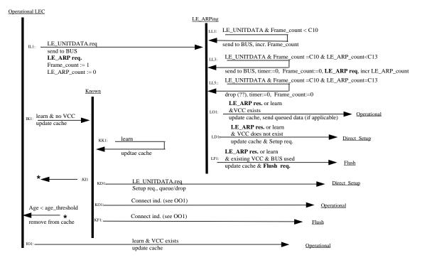
Figure 13. LAN Destination State Machines (LE\_ARP)
