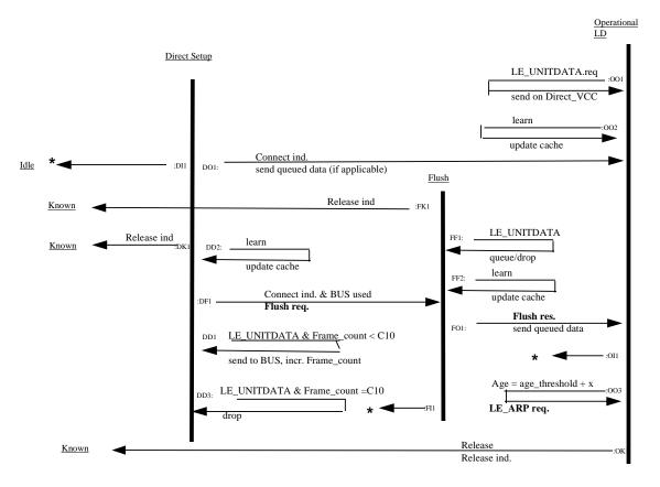
Figure 14. LAN Destination State Machines (Direct Setup)
