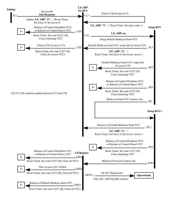
Figure 11. LE Client State Machine (Join, LE\_ARP)
