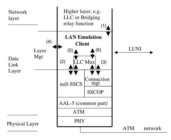
Figure 1. The Layered Architecture of LAN Emulation
