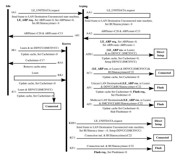
Figure 14. LAN Destination State Machines (Part 1)
