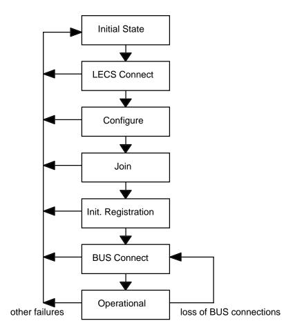
Figure 8. Initialization, Recovery and Terminating the ELAN
