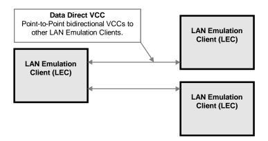
Figure 6. LAN Emulation Client to Client Data Connections
