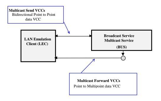
Figure 7. LAN Emulation Client Broadcast/Multicast Connections
