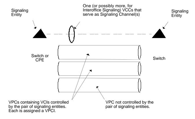
Figure 1-4 Signaling Channel(s) and VPCs Used as Bearer Channels
