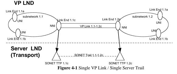
The ATM Link points to two different instance of the ATM Link End. Each ATM Link End points to an entity that represents the underlying server trail termination. Information associated with the specific interface is included in the ATM Link End at the VP LND. Optionally, the ATM Link End may include server layer termination point specific information.
