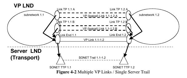
In the following example, a single VP Link is supported by multiple underlying server trails (and multiple topological links). The VP Logical Link TP has a continuous range of VPI values, where the underlying ATM Link End related ranges are non-overlapping. Total logical link bandwidth is the sum of the topological links bandwidth.
