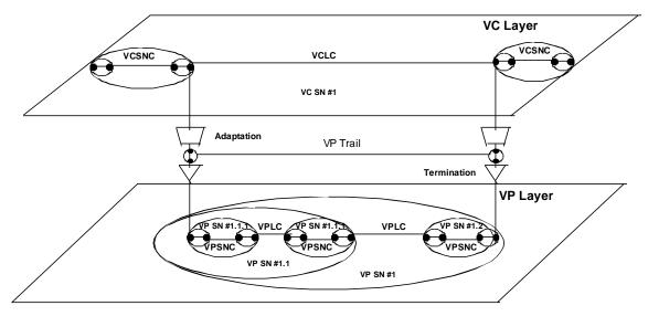
SN: SubNetworkSNC: SubNetwork ConnectionLC: Link Connection
