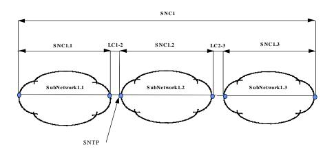
Figure 6.3.2.2-a: Network Transport Architecture
