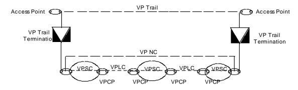
Figure 2 ATM VP Layer Network
