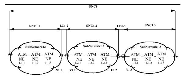
Figure 6.2.3.2-a: Network Transport Architecture
