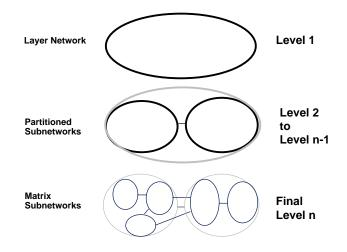
Figure 1 Example of subnetwork Partitioning
