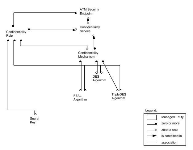
Figure 4-2: Managed Entity Relationship Diagram for the Confidentiality Service
