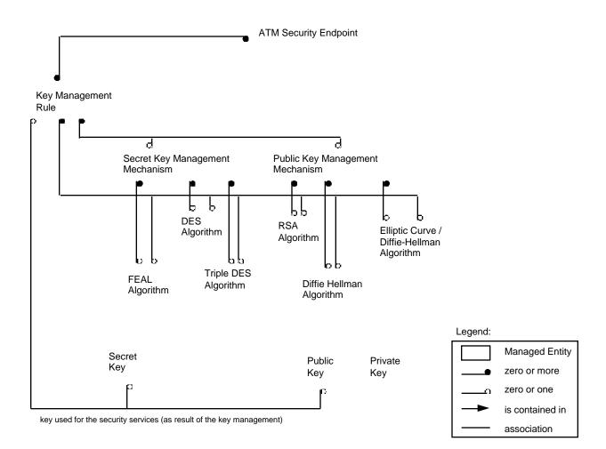
Figure 4-4 : Managed Entity Relationship Diagram for Key Management
