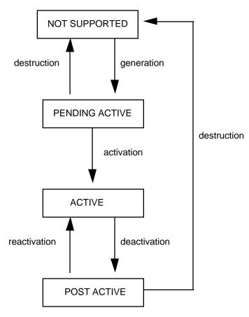
Figure 3-3: Life cycle state diagram
