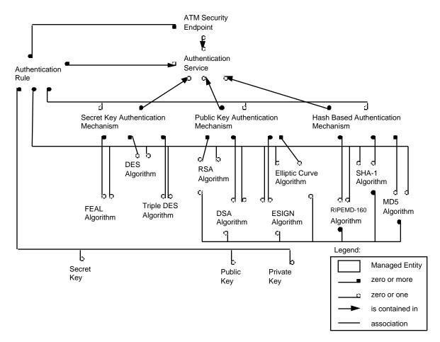
Figure 4-1: Managed Entity Relationship Diagram for the Authentication Service
