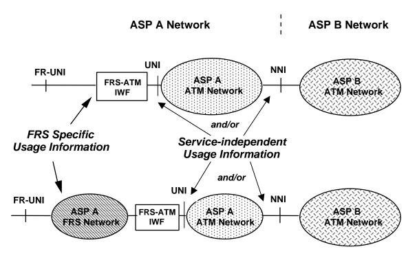
Figure 3-3 PVC FRS Usage Measurements
