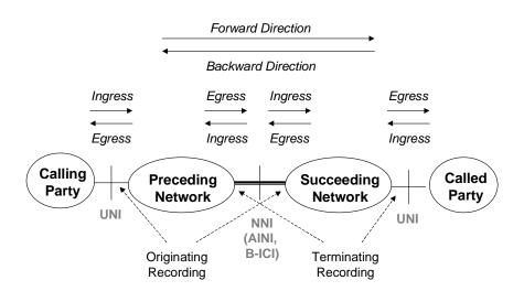
Figure 4-1 SVC Usage Measurement Reference Model – Network View
