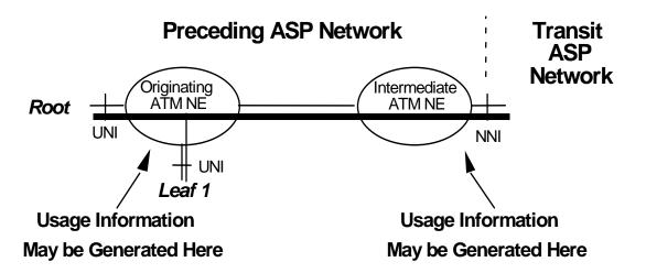
Figure C-2 Point-to-Multipoint SVC Recording in the Preceding ASP Network
