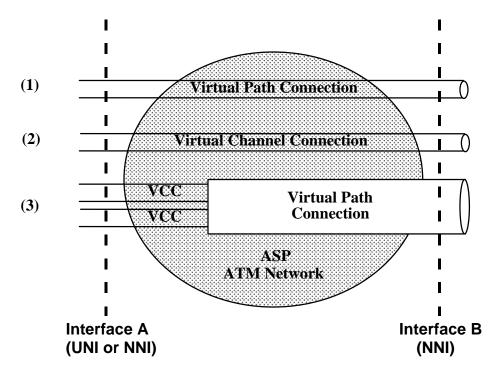
Figure 2-1 Examples of PVC Configurations
