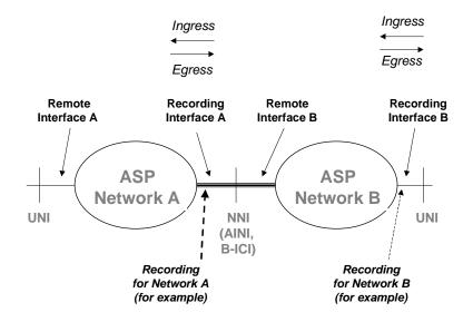
Figure 2-2 PVC Usage Measurement Reference Model
