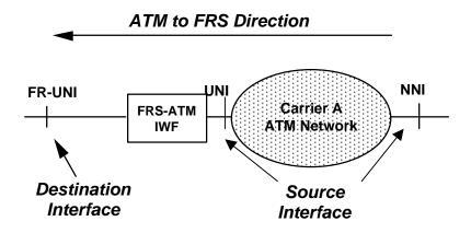
Figure 3-4 Types of Interfaces for PVC FRS Usage Measurement
