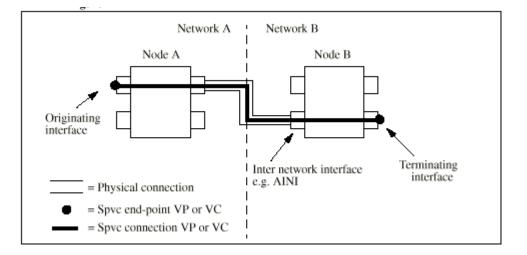
Figure 5-1 SPVC Usage Measurement Reference Model
