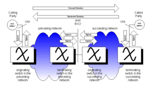
Figure 4-2 SVC Usage Measurement Reference Model – Switch View
