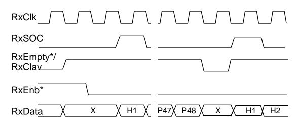
Figure 7. RxEmpty\*/RxClav Timing
