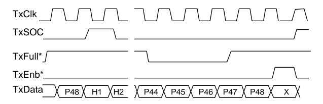
Figure 4. Transmit Timing for Cell-Level Handshake
