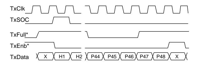
Figure 3. Transmit Timing for Octet-Level Handshake
