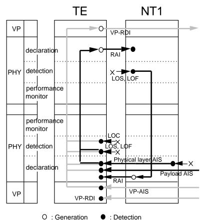
Figure 2-4 Maintenance signal flow
