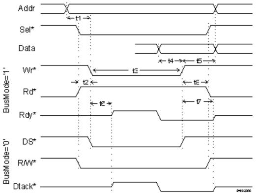
Figure 3.2: Single data byte write transfer (parallel interface)
