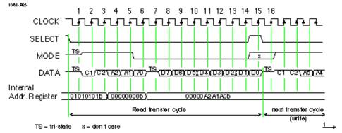
Figure 2.2: Single data byte read transfer
