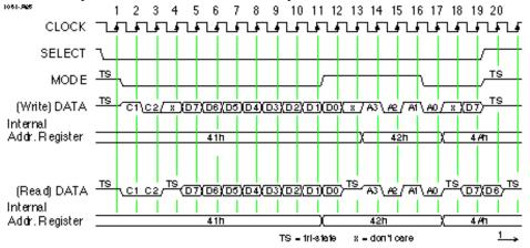
Figure 2.4: Multiple data byte write (read) transfer (aborted)
