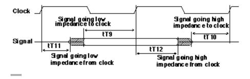
Figure 2.6: Tri-state timing definition (serial management interface)
