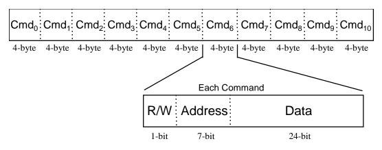
Figure 5.10: Register Read/Write Message
