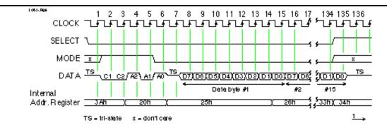
Figure 2.3: Multiple data byte read transfers (successive byte locations)
