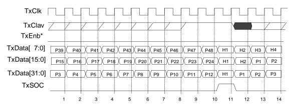
Figure 3.1: Transmission of two cells back-to-back
