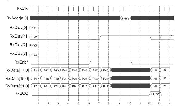
Figure 4.6: PHY layer device not ready to send cell
