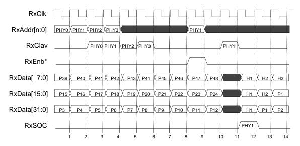
Figure 4.10: Receive Decode and Selection
