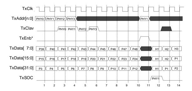
**Figure 4.8: Transmit Decode and Selection**
