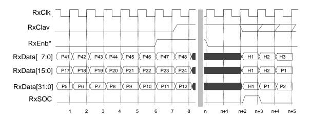
Figure 3.6: PHY layer device not ready to transmit cell
