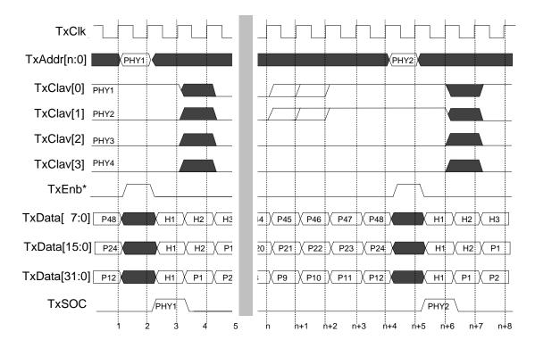
Figure 4.1: Transmit Decode and Selection
