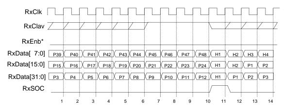
Figure 3.4: Reception of two cells back-to-back
