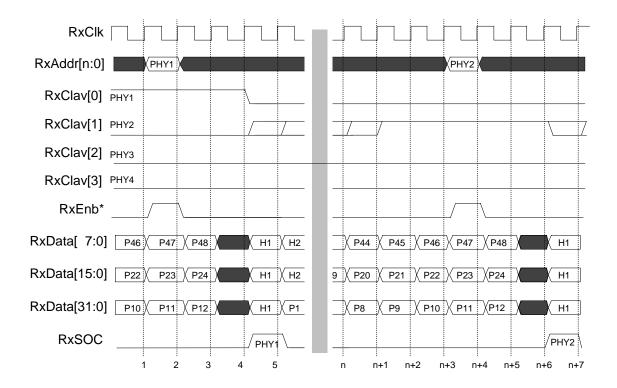
**Figure 4.4: Receive Decode and Selection**
