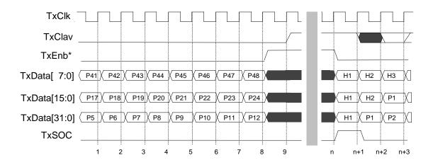
Figure 3.3: PHY layer device not ready to receive cell
