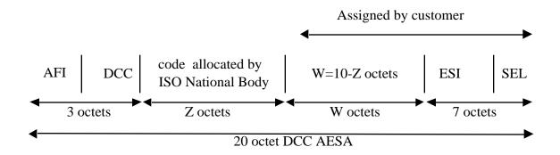
Figure 4-3: Example of a DCC Customer Owned AESA
