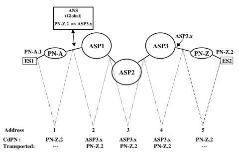
Notes: ASP1, ASP2 & ASP3 route on address ASP3.x but not on address PN-Z.2. ASP3.x is an ATM WAN address, and PN-Z.2 is an ATM Local (User) address.
