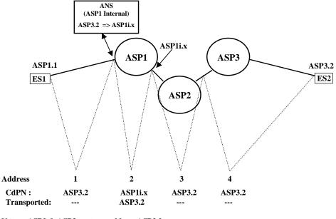
Notes: ASP2 & ASP3 route on address ASP3.2. But ASP1, an Internally Addressed Network, does not route on ASP3.2. For ASP1, ASP3.2 is an ATM External Address, and ASP1i.x is an ATM Internal Address
