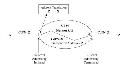
Figure 3-1 ATM Bi-Level Addressing Concept
