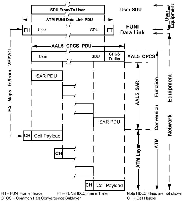
Figure 3.1 Encapsulation/Decapsulation and ATM Conversion Process for AAL5 (Physical Layer is Not Shown in This Diagram)
