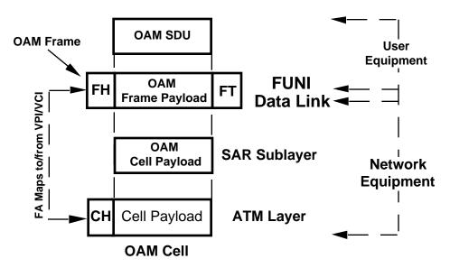
Figure 5.1 Cell-to-Frame Mapping of Management Cells
