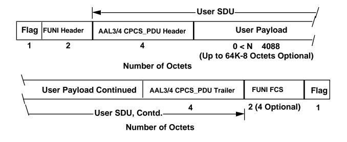
Figure 3.4 Illustration of the AAL3/4 User SDU and FUNI PDU (AAL3/4 CPCS\_PDU)
