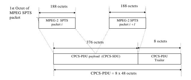
Figure 6 Format of AAL-5 PDU Containing 2 TS Packets
