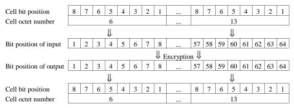
Figure 38: SymmetricEncryption Algorithm Data Bit Ordering.
