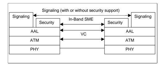
Figure 18: Access Control Layer Reference Model for In-Band-Based Messaging.
