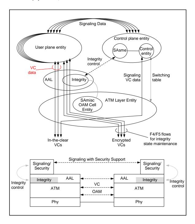
Figure 14: Object and Layer Reference Models for Data Integrity with Signaling-Based SME.
