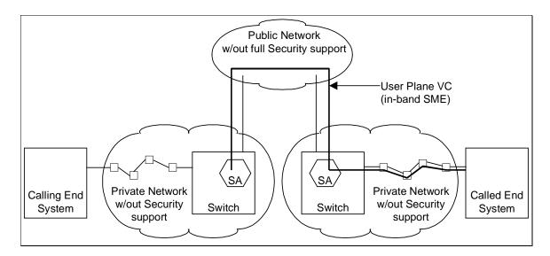
Figure 9: Using the In-Band SME Protocol in Networks that do not support Signaling-Based SME.
