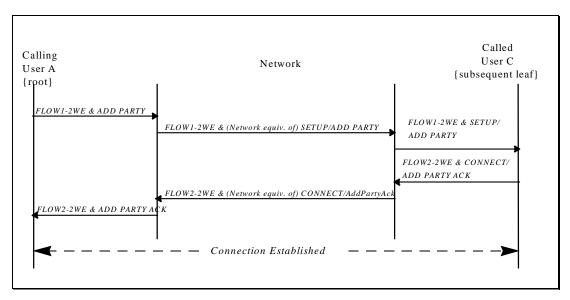
Figure 23: Point to Multipoint Signaling Support for Two-Way Security Message Exchange for Subsequent Leaf Setup.
