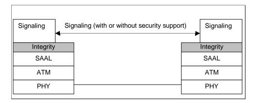
Figure 19: Control Plane Data Origin Authentication and Integrity Layer Reference Model.
