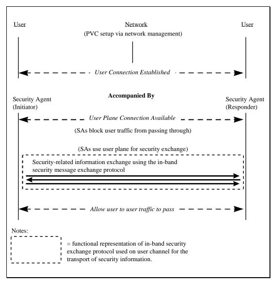
Figure 25: Point-to-Point Security Exchange using the Hosts' User Plane for PVCs.
