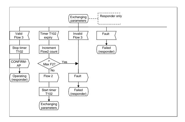
Figure 37: Detailed SDL for Three-Way SME Initiator and Responder Procedures.
