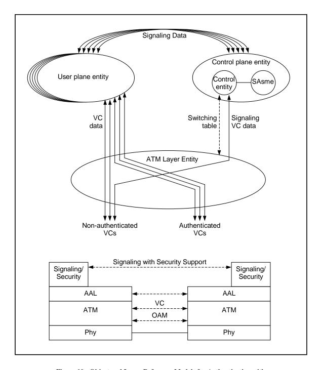
Figure 10: Object and Layer Reference Models for Authentication with Signaling-Based SME.
