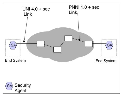
Figure 7: Entire Network Supports Signaling-Based SME.
