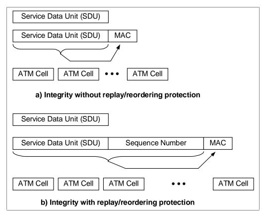
Figure 16: AAL-SDU Level Data Integrity.
