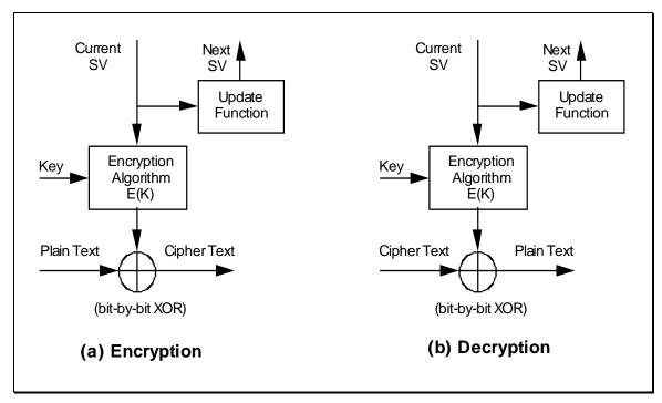
Figure 40: Counter Mode Block Diagram.
