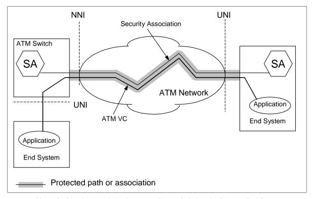
Figure 3: Security Association between a SA at a Switch and a SA at an End System.
