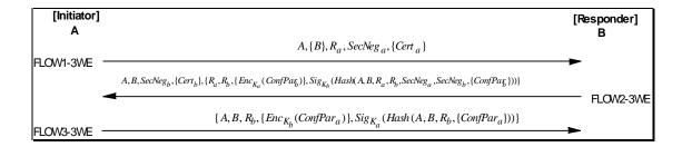
Figure 20: Three-Way Security Message Exchange Protocol.
