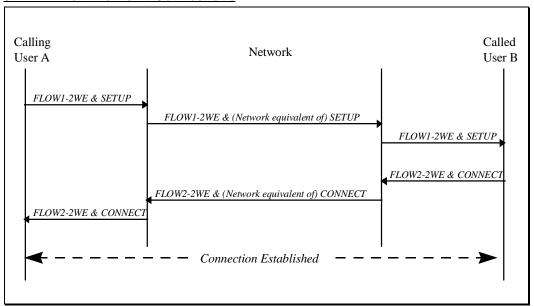
Figure 22: Point-to-Point Signaling Support for Two-Way Security Message Exchange.
