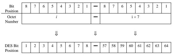
Figure 39: Symmetric Encryption Algorithm Key Bit Ordering.
