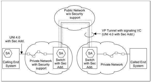
Figure 8: Portion of Network Does Not Support Signaling-Based SME.
