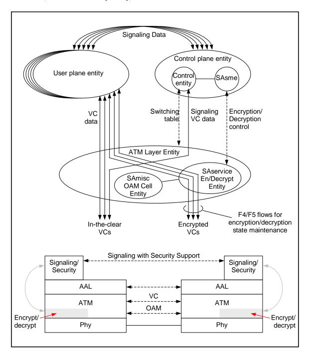
Figure 12: Object and Layer Reference Models for Confidentiality with Signaling-Based SME.
