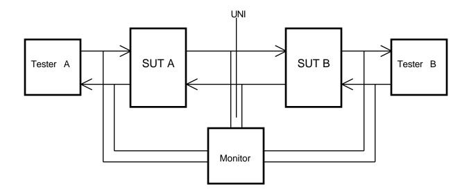
Figure 3.2: Test Configuration #1
