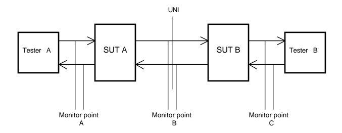
Figure 3.1: Generic ATM Layer Test Configuration
