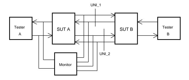
Figure 3.7: Test Configuration #6 (Note: UNI\_1.... UNI\_2 are located on separate physical links)
