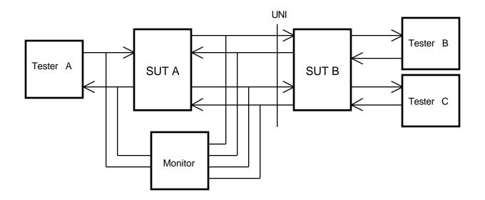
Figure 3.6: Test Configuration #5 (Note: the VPC or VCC created may be on the same or different physical link)
