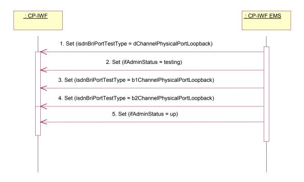
Figure 7: Procedure for carrying out loopback tests
