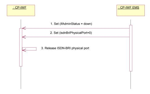
Figure 6: Procedure for releasing a physical port assigned to a CP-IWF user port
