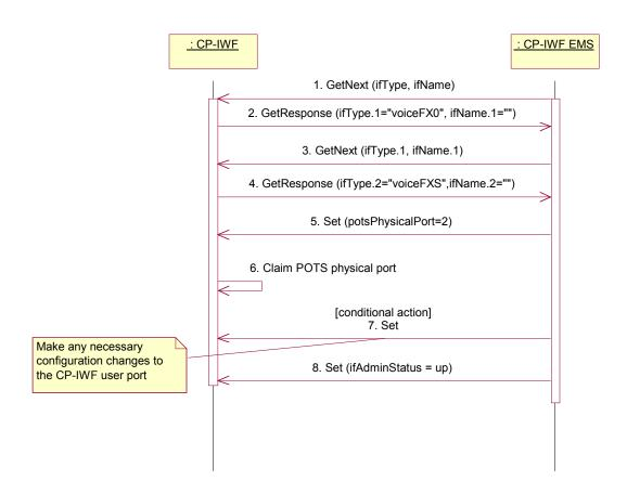
Figure 5: Procedure for assigning a physical port to a CP-IWF user port
