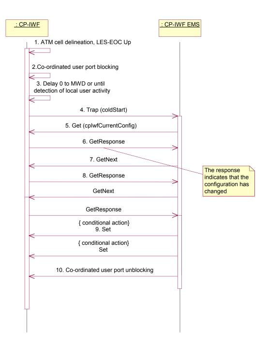
Figure 4: Procedure for CP-IWF Start-up/Restart
