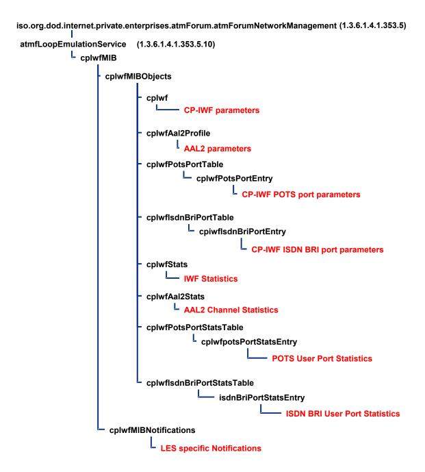
Figure 3. Structure for Configuration MIB
