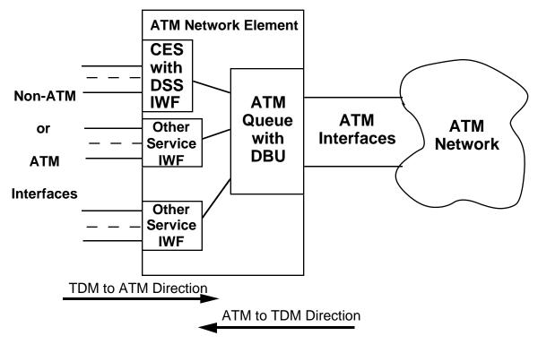
DSS = Dynamic Structure Sizing DBU = Dynamic Bandwidth Utilization
