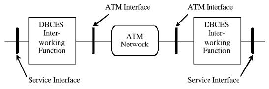
Figure 5.1: Reference Network Configuration
