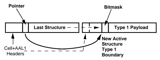
Figure 3.3 Illustration of the Beginning of a Type 1 Active Structure
