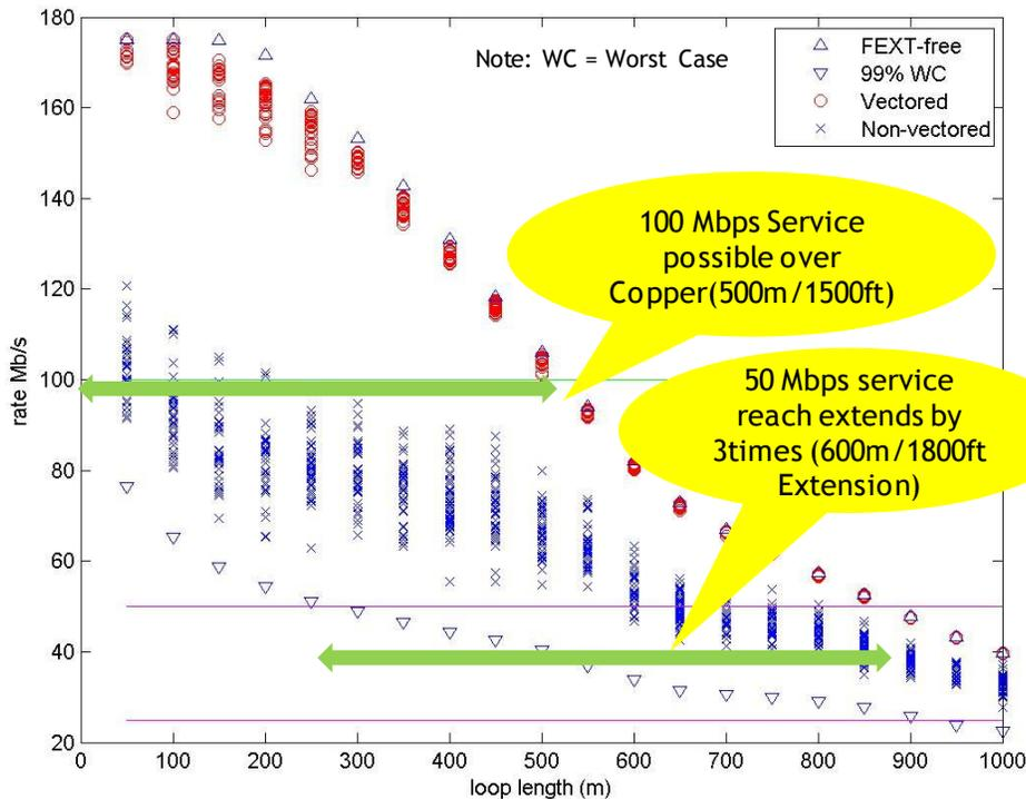
**Figure 6 - Downstream Rates – Profile 17a, 26 AWG, -136 dBm/Hz noise, 80 users, and 47 cancelled**
