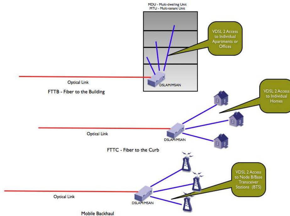
**Figure 9 - Schematic of Deployment Architectures**
