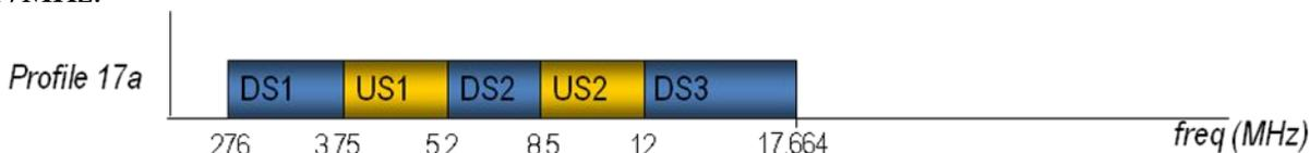
Figure 5 - Example band plans for profile 17a
