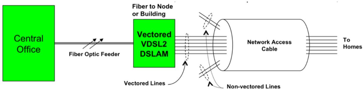
**Figure 2** - Reference Fiber Fed DSL Network Access Architecture
