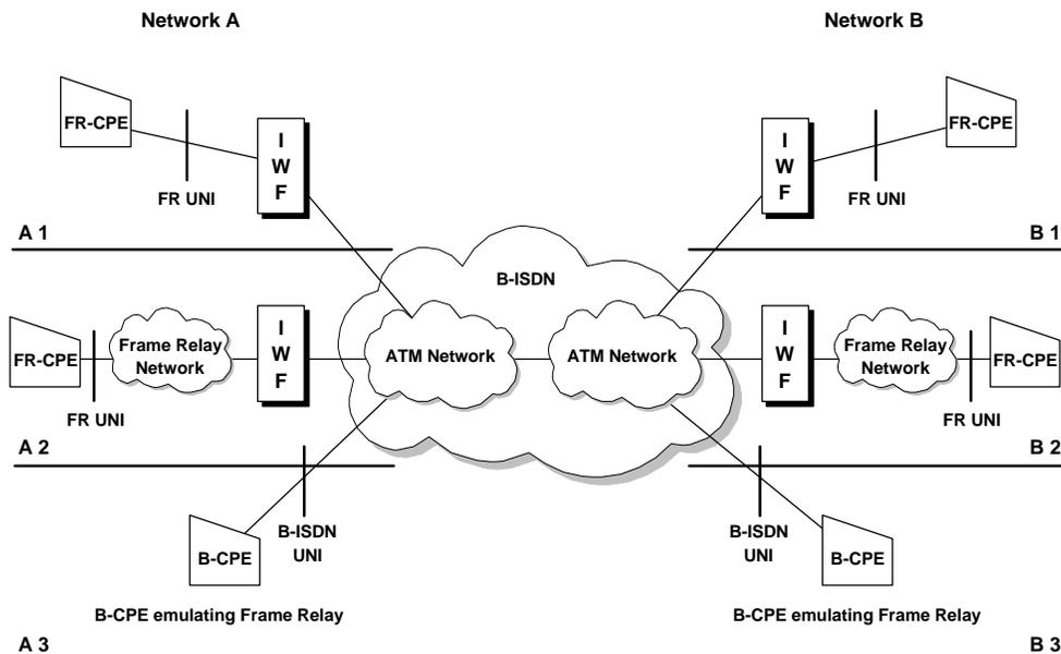
**Figure 1: FRS Support on an ATM-based Multi-Service Interface**
