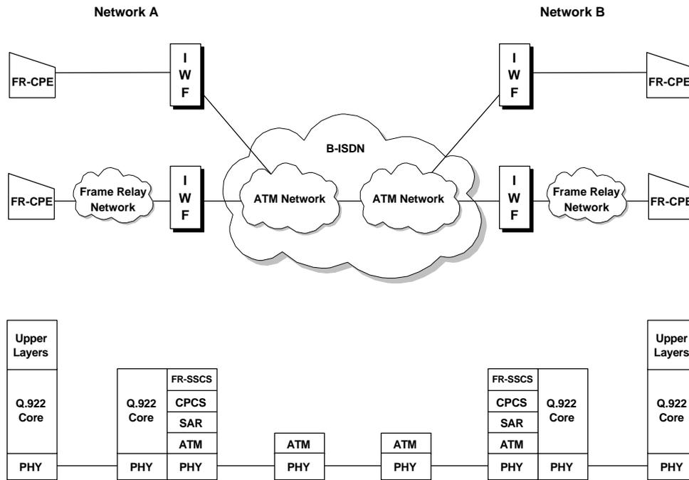
**Figure 3: Network Interworking between FRBS and B-ISDN**
