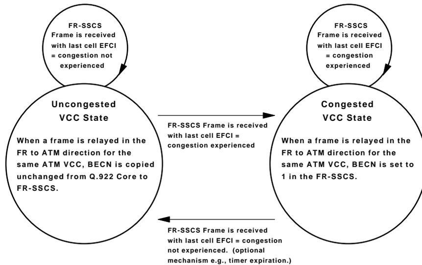
Figure 10: Congestion State Diagram for VCC
