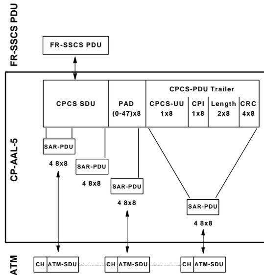
**Figure 7: Common Part AAL-5 PDU Formats**
