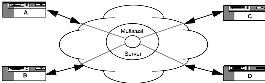
Figure 4. - N-Way Multicast
