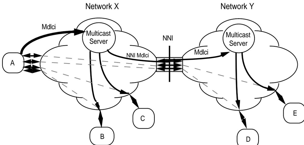
**Figure 6 - One-way Multicast across an NNI**
