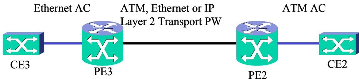
**Figure 4 ATM-Ethernet Interworking over MPLS**
