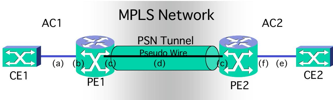
**Figure 1 Defect Model for Multi-service interworking**
