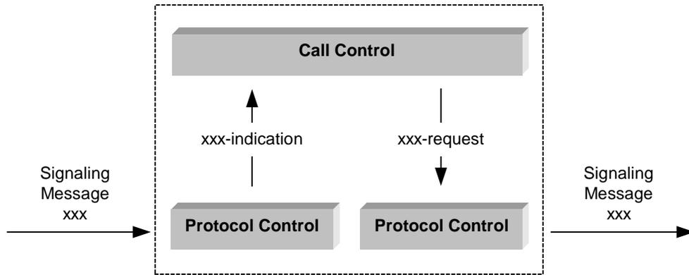
**Figure 1-1 Primitives used in the NCCI procedures**
