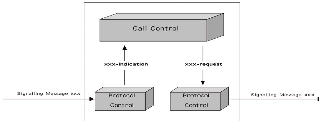
Figure 4-2: Primitives used in the Signalling specification sections
