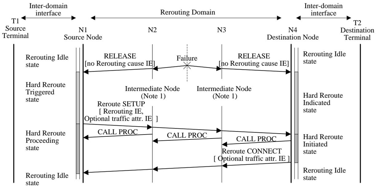
Note 1: Intermediate Node which is part of the "rerouting" connection path.
