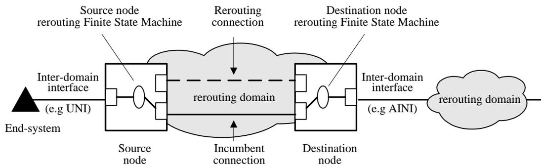
Figure 4-1: Operational model of domain-based rerouting
