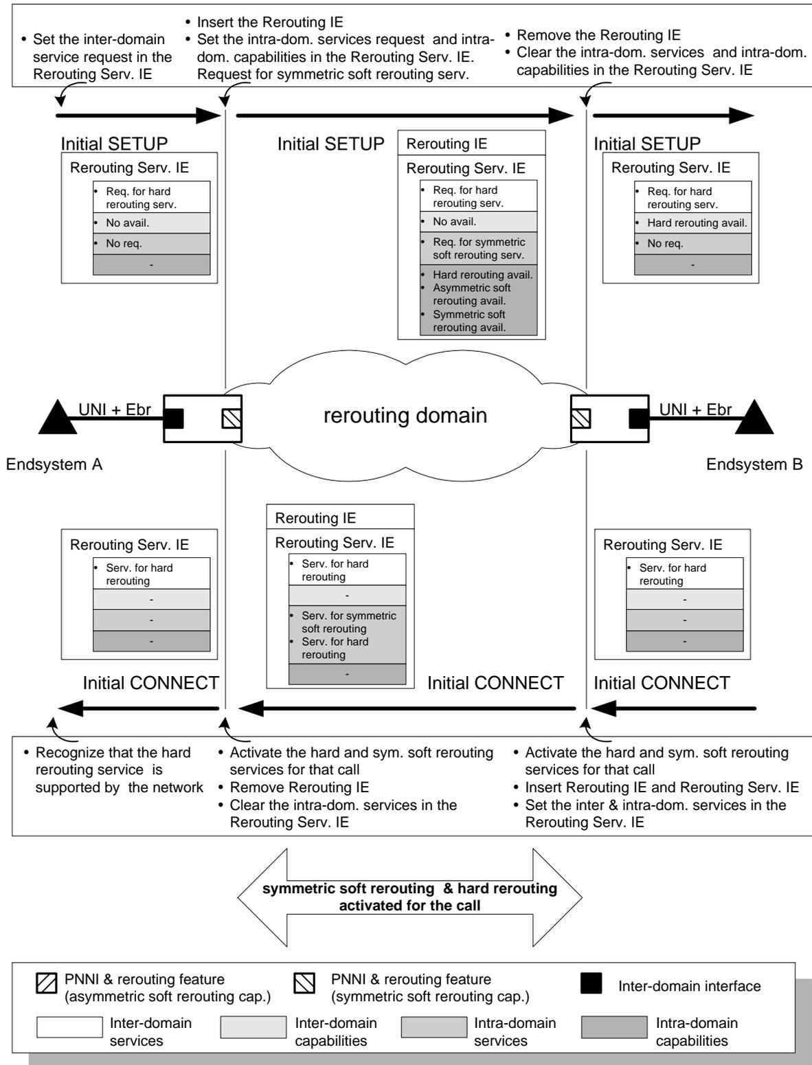
Figure Appendix D-4: Negotiation of the rerouting services over one rerouting domain. Hard rerouting requested by the calling end system. Asymmetric soft rerouting requested by the source node.
