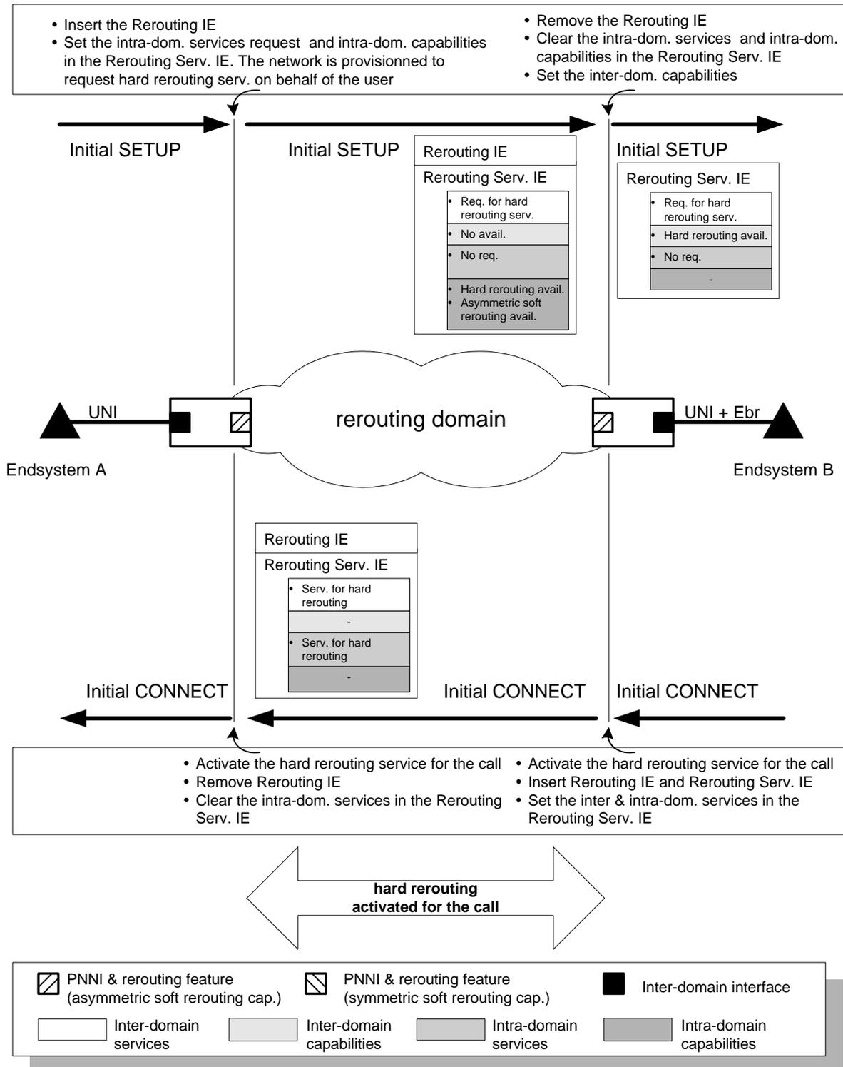
Figure Appendix D-2: Negotiation of the rerouting services over one rerouting domain. Hard rerouting requested by the source node on behalf of the end system.
