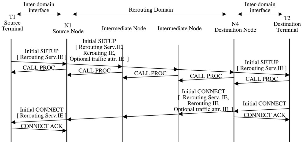
Figure 4-8: Flow Sequence during the initial connection establishment over a single rerouting domain
