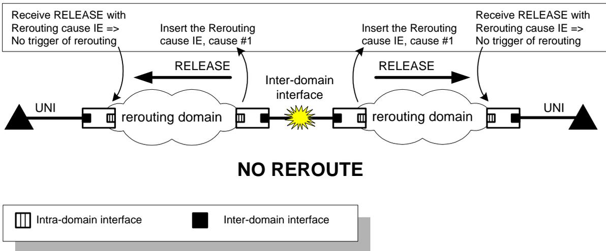
Figure 4-6: Edge switch inserts the Rerouting cause information element to indicate no trigger for rerouting
