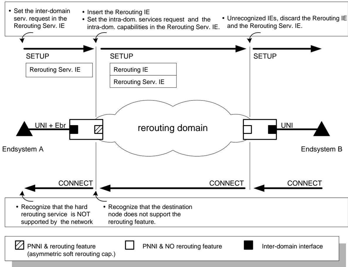
Figure Appendix D-6: Negotiation of the rerouting services over one rerouting domain. The destination node does not support the rerouting feature
