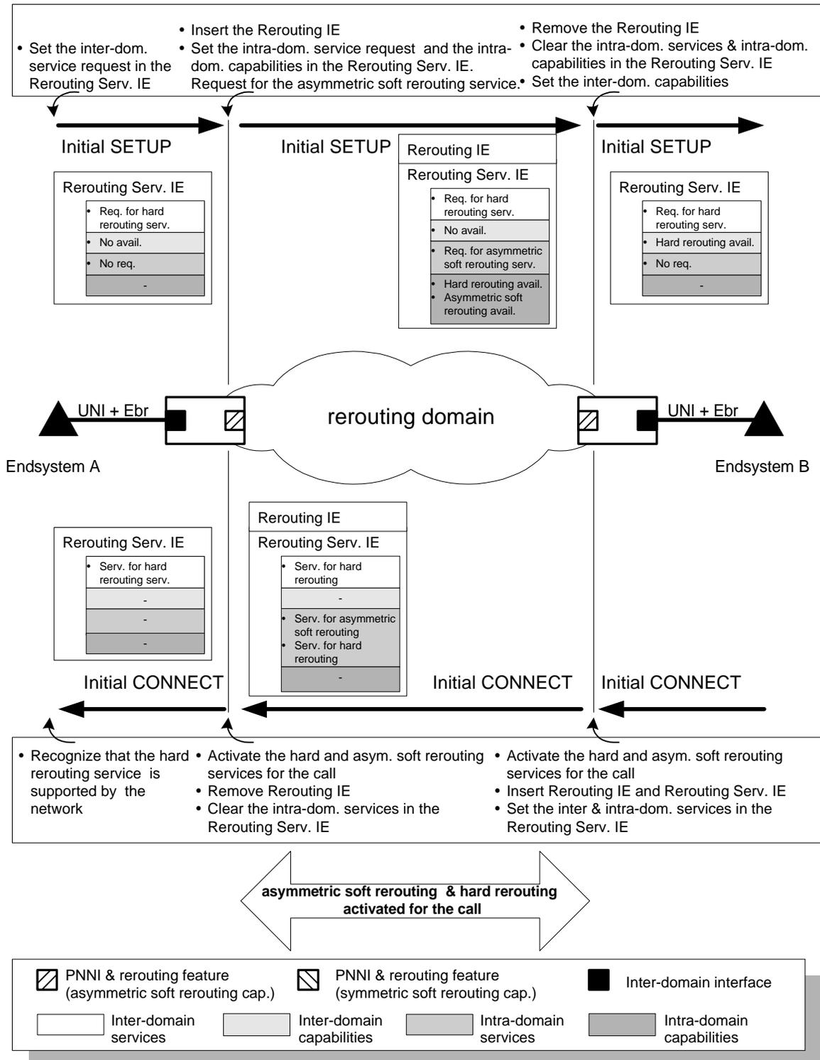
Figure Appendix D-1: Negotiation of the rerouting services over one rerouting domain. Hard rerouting requested by the calling end system. Asymmetric soft rerouting requested by the source node.
