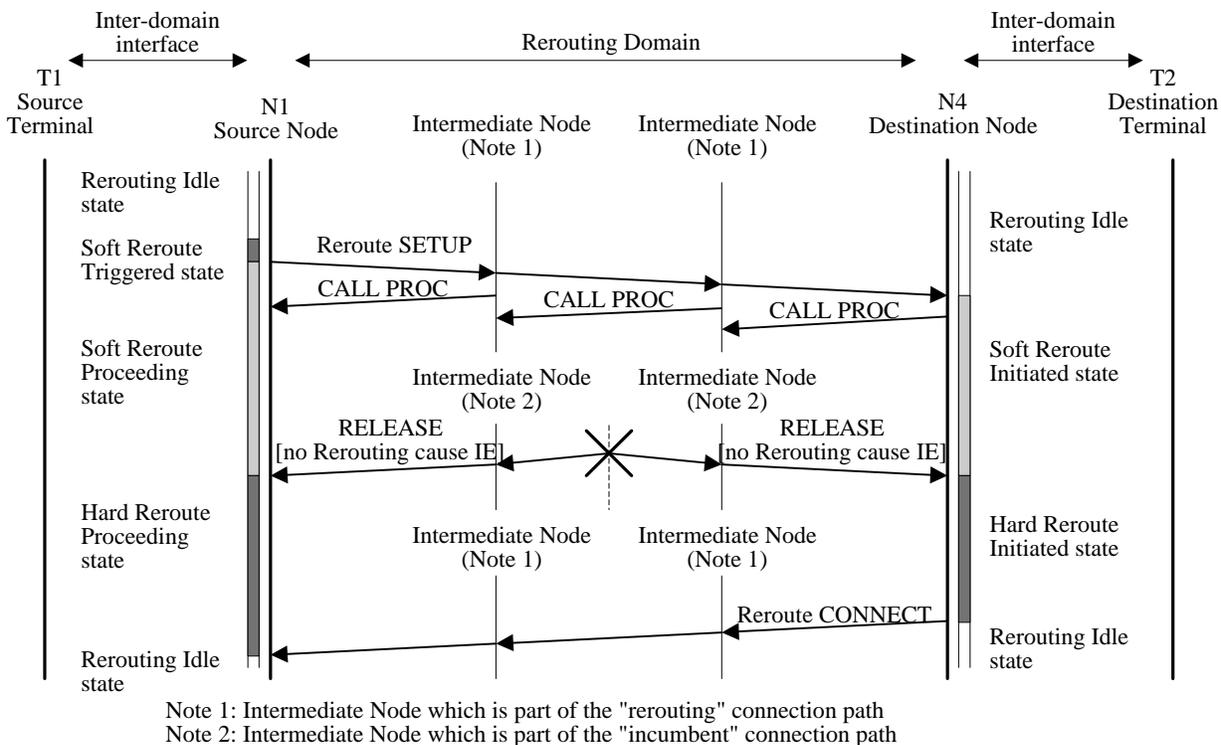
Figure 4-14: "Incumbent" connection failed during soft rerouting
