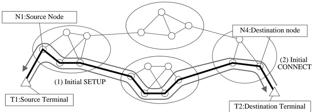
Figure 4-7: Initial connection establishment over a single rerouting domain
