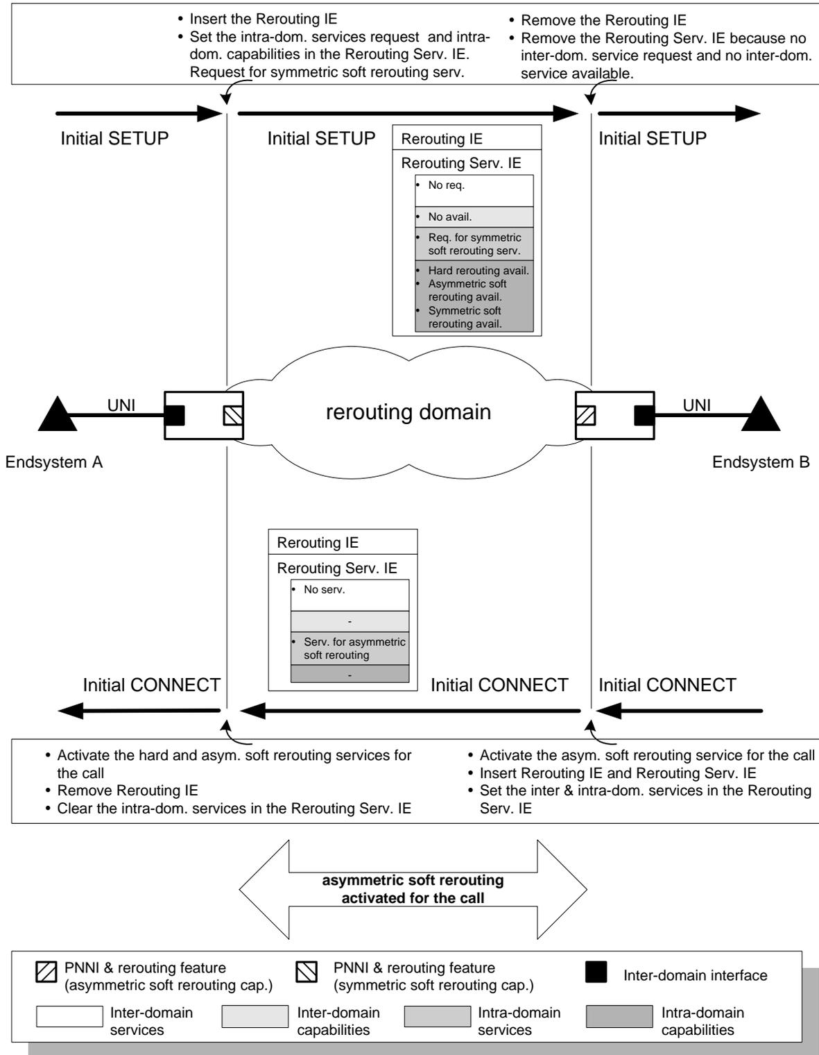
Figure Appendix D-5: Negotiation of the rerouting services over one rerouting domain. The destination node does not support symmetric soft rerouting
