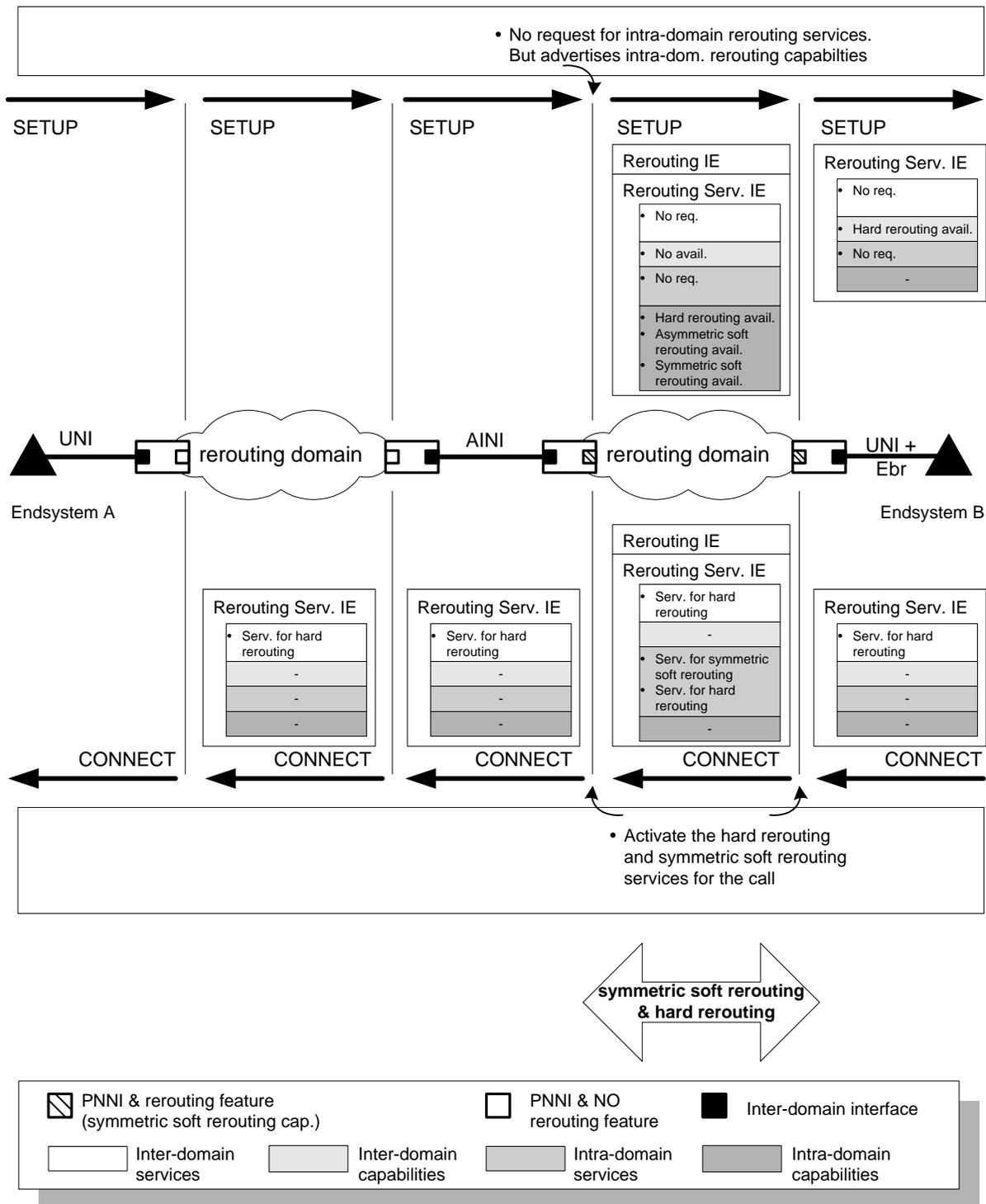
Figure Appendix D-8: Negotiation of the rerouting services over two rerouting domains. Hard rerouting requested by the called end system. Symmetric soft rerouting requested by the destination node of the second rerouting domain.
