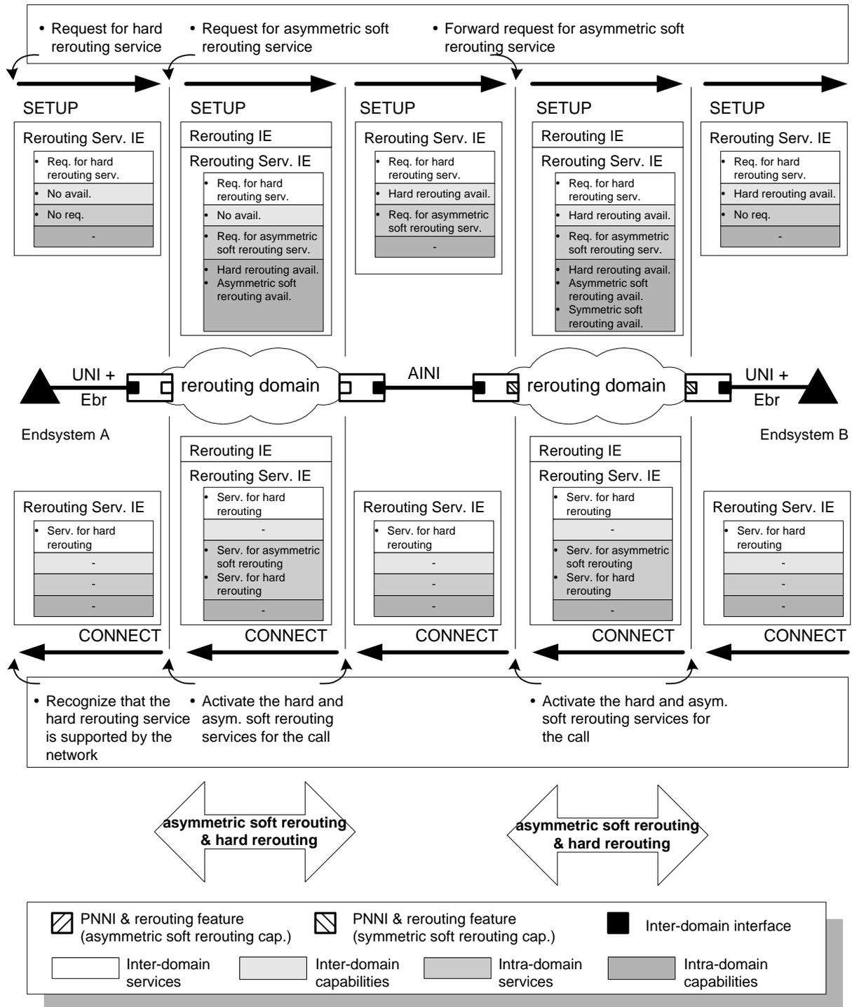
Figure Appendix D-7: Negotiation of the rerouting services over two rerouting domains. Hard rerouting requested by the calling end system. Asymmetric soft rerouting requested by the source node of the first rerouting domain and passed to the second rerouting domain.
