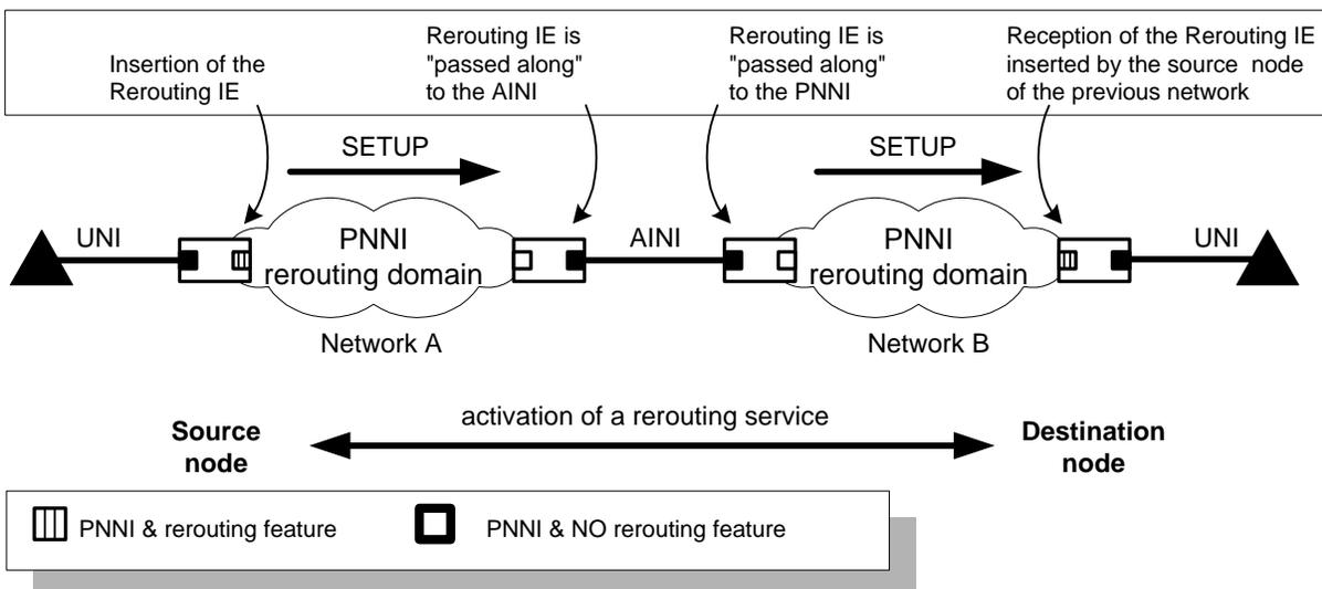
Figure 10-1: Incorrect association between the source node and the destination node when a call spans over multiple rerouting domains
