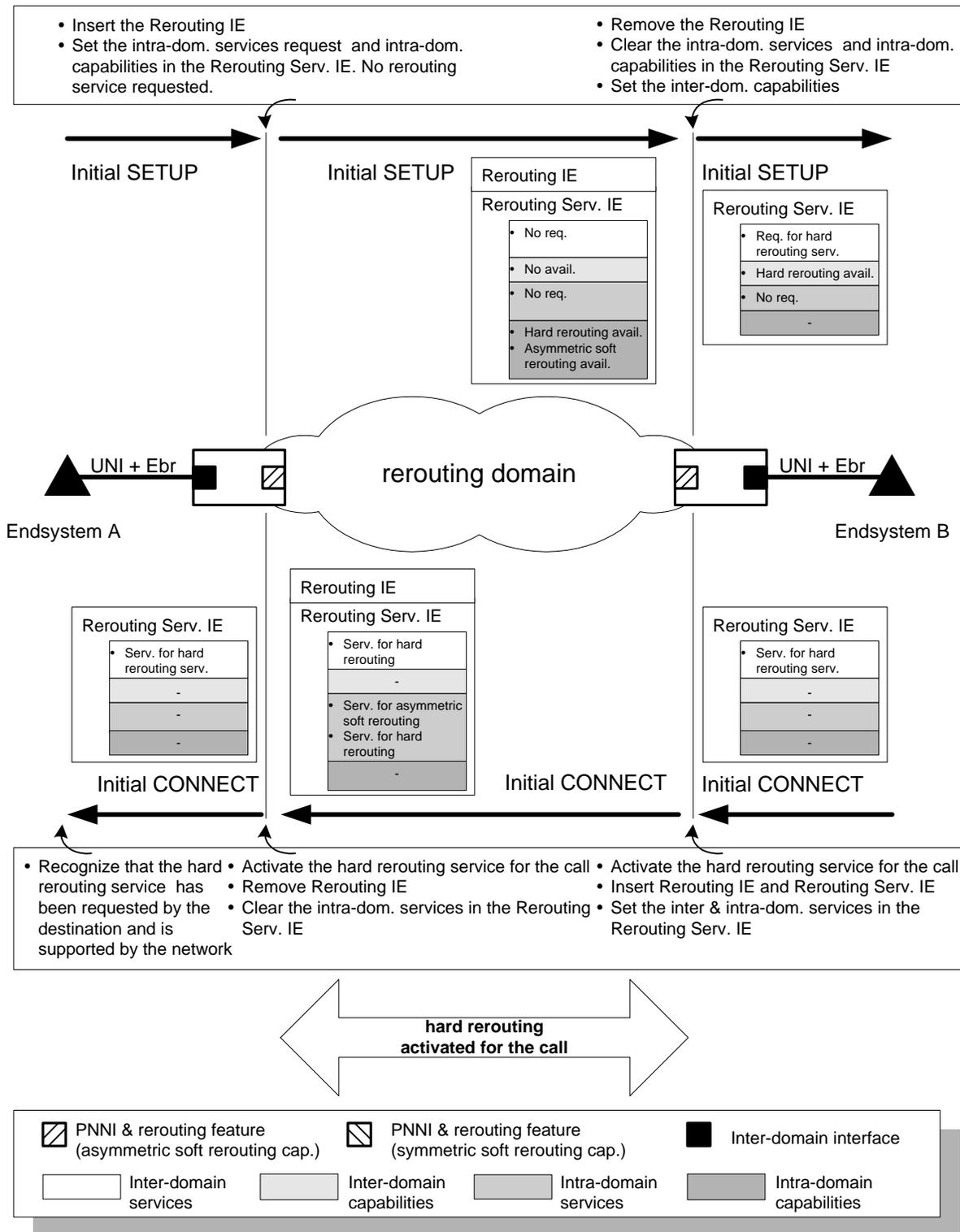
Figure Appendix D-3: Negotiation of the rerouting service over one rerouting domain. Hard rerouting requested by the called end system.
