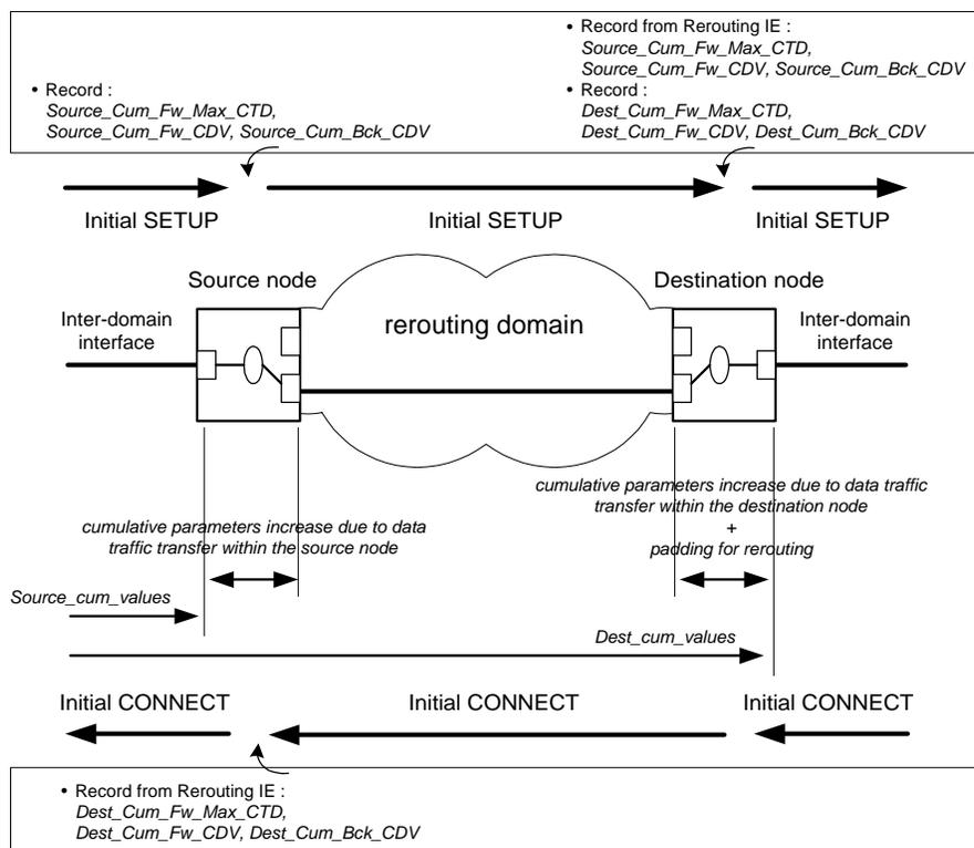
Figure Annex A-1: Exchange of the cumulative parameters between the source node and the destination node during the initial call establishment
