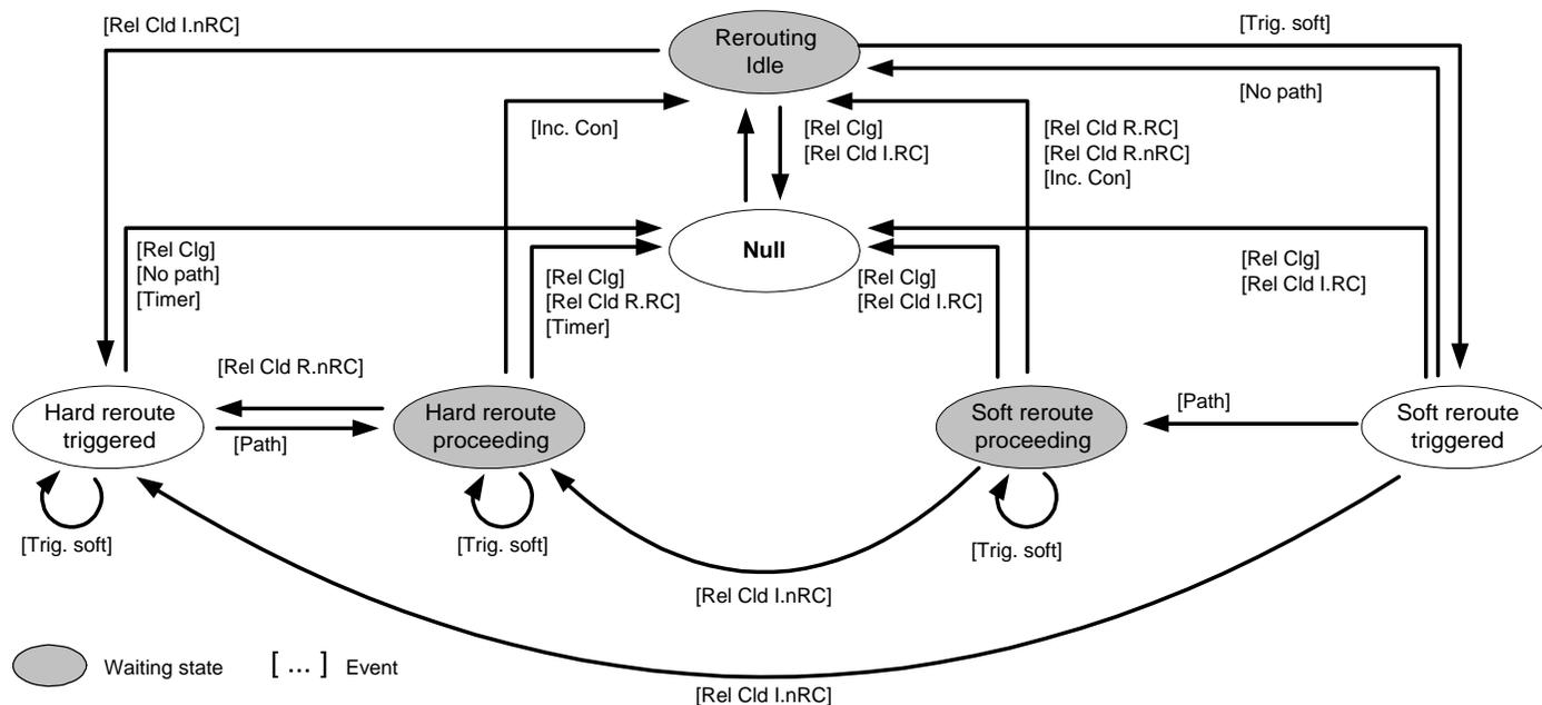
Figure Appendix B-1: Rerouting state transitions at the source node (hard and asymmetric soft rerouting)
