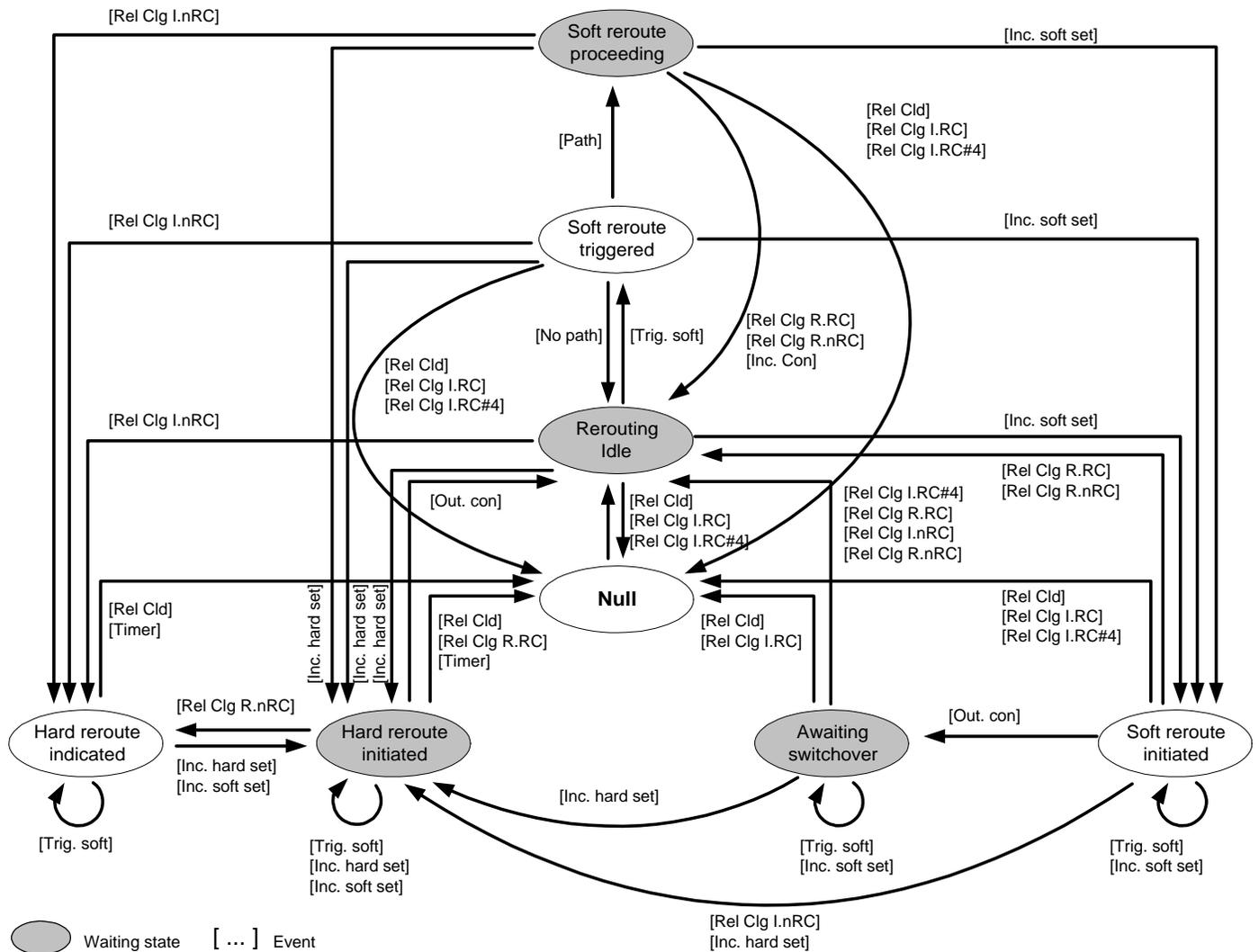
Figure Appendix C-2: Rerouting state transitions at destination node (hard and symmetric soft rerouting)
