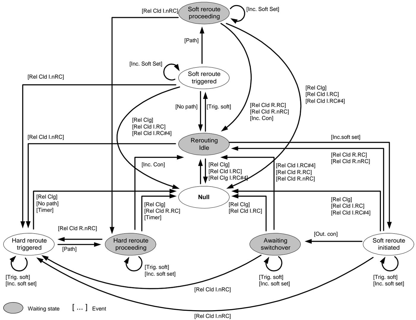
Figure Appendix C-1: Rerouting state transitions at the source node (hard and symmetric soft rerouting)
