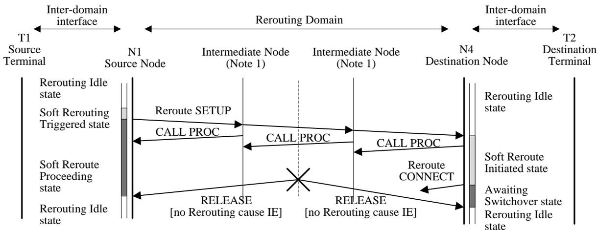
Note 1: Intermediate Node which is part of the "rerouting" connection path
