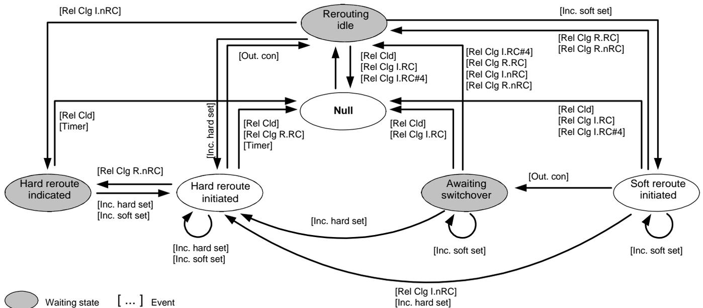
Figure Appendix B-2: Rerouting state transitions at the destination node (hard and asymmetric soft rerouting)
