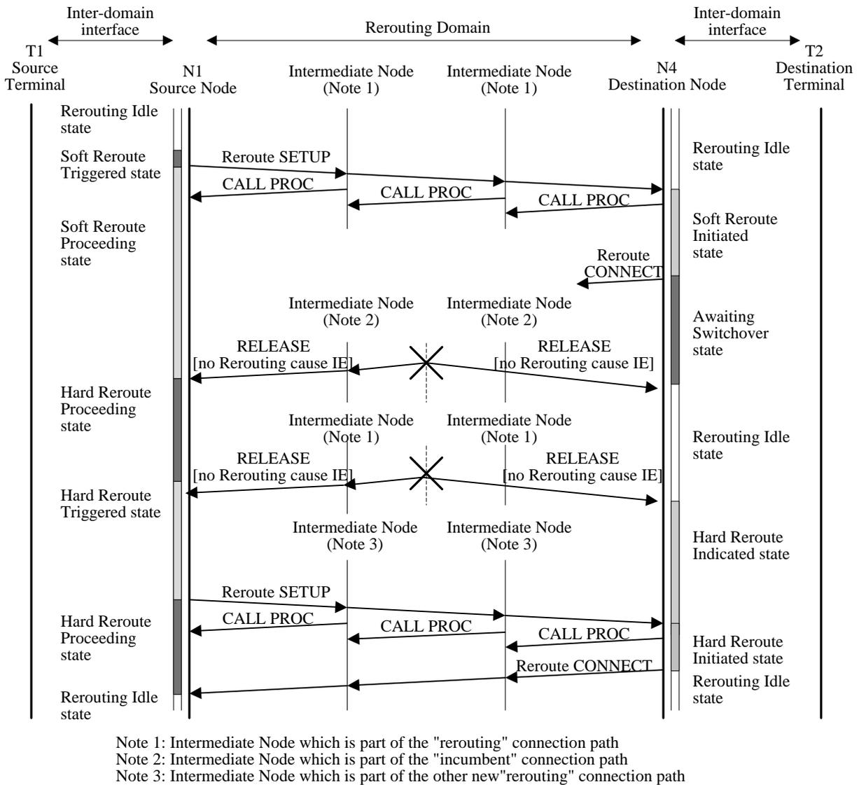
Figure 4-15: "Rerouting" connection failed after "Incumbent" connection failed during soft rerouting
