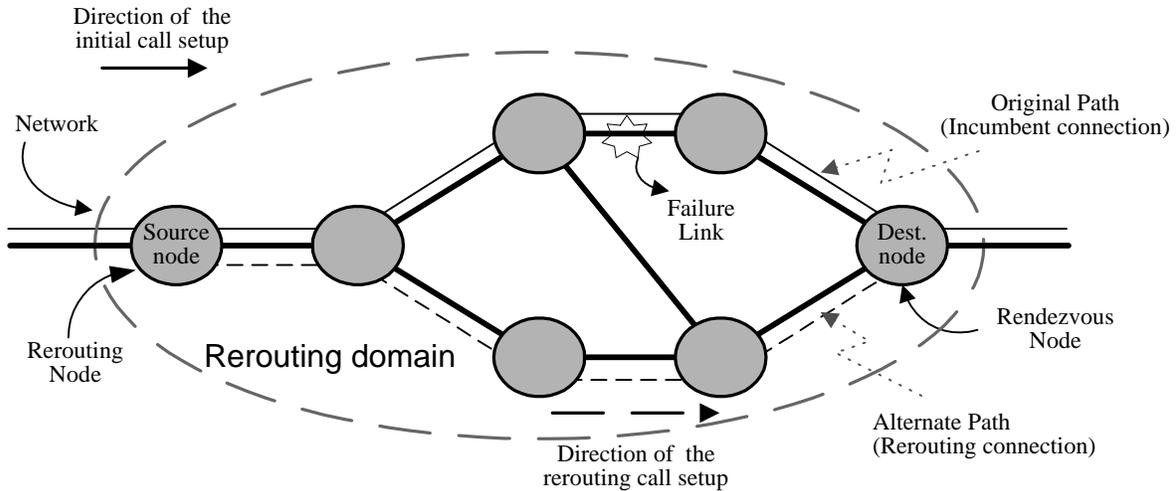
Figure 2-1: Hard rerouting example
