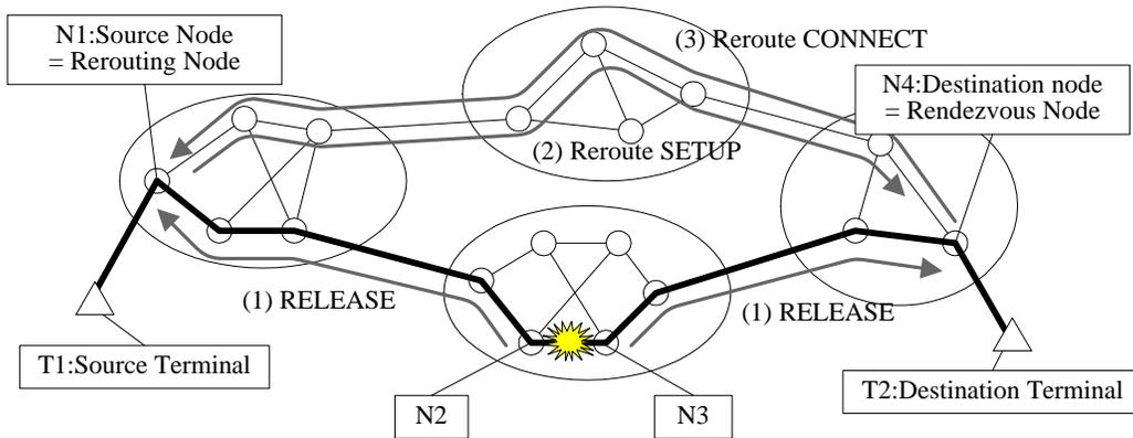
Figure 4-9: Hard rerouting operation
