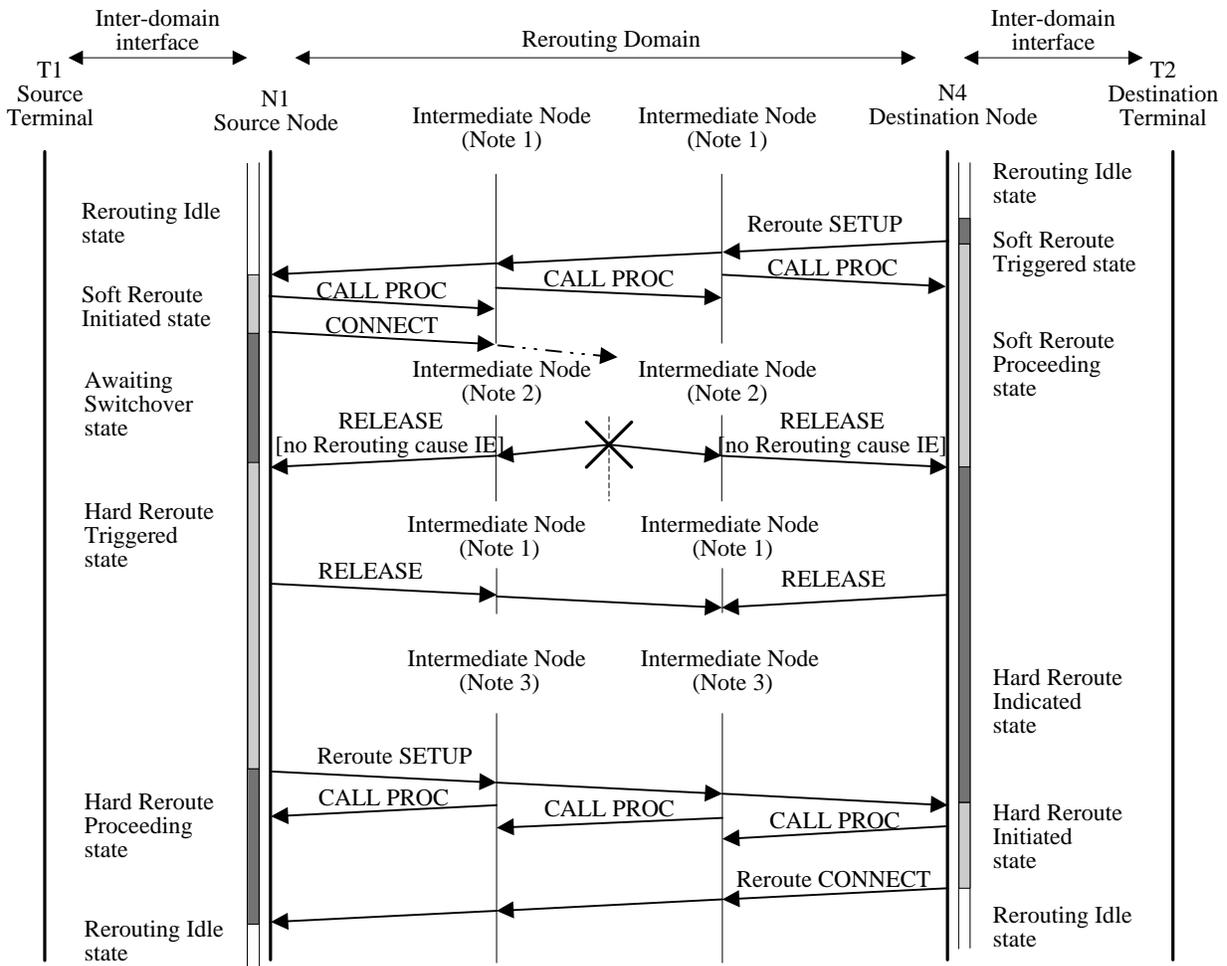
Note 1: Intermediate Node which is part of the "rerouting" connection path
