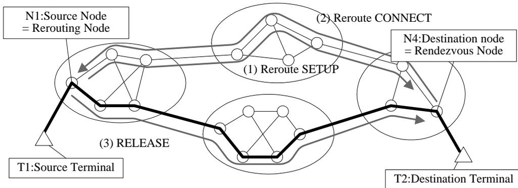
Figure 4-11: Soft rerouting operation
