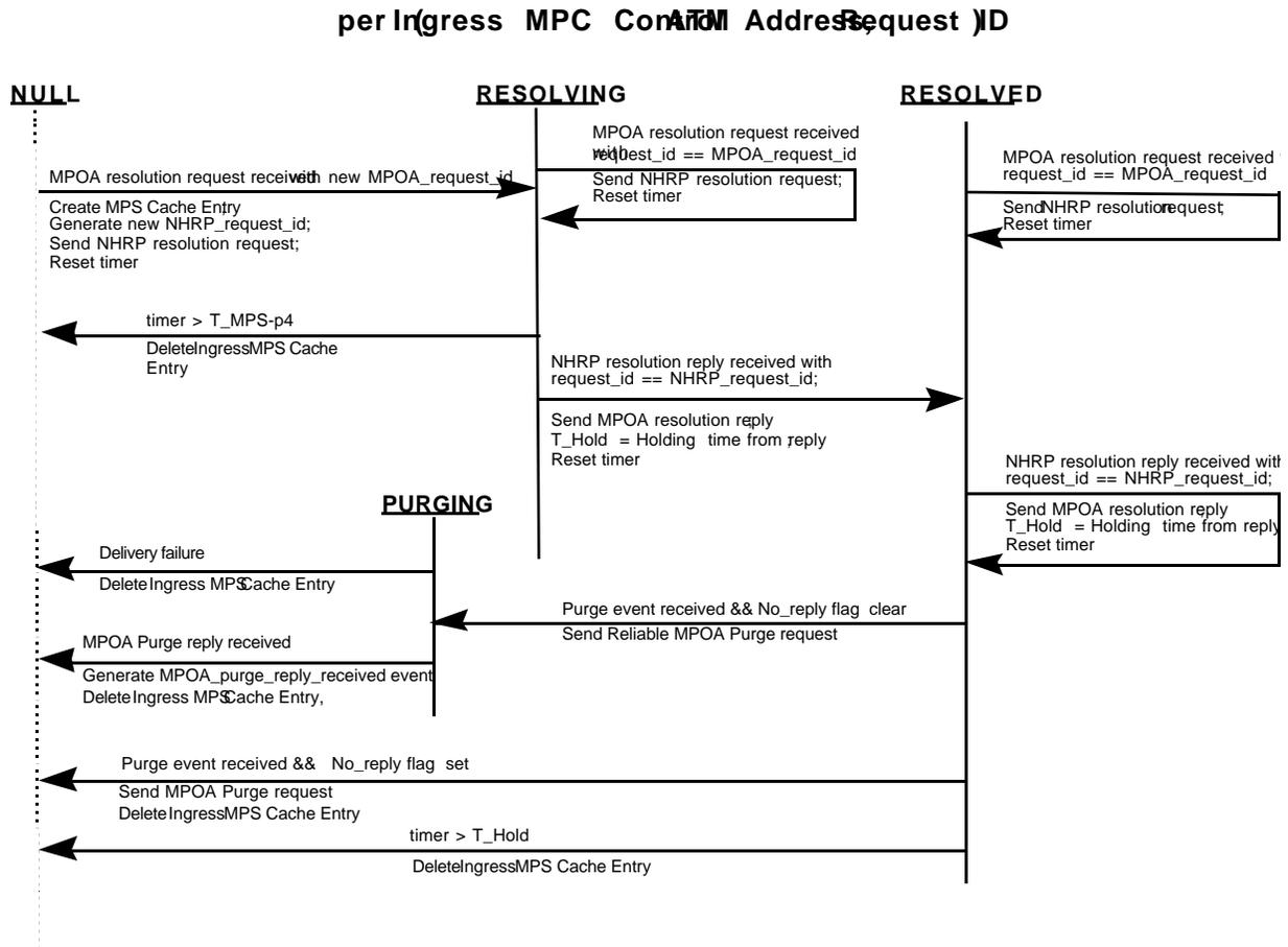
Figure 24 Ingress MPS Control State Machine
