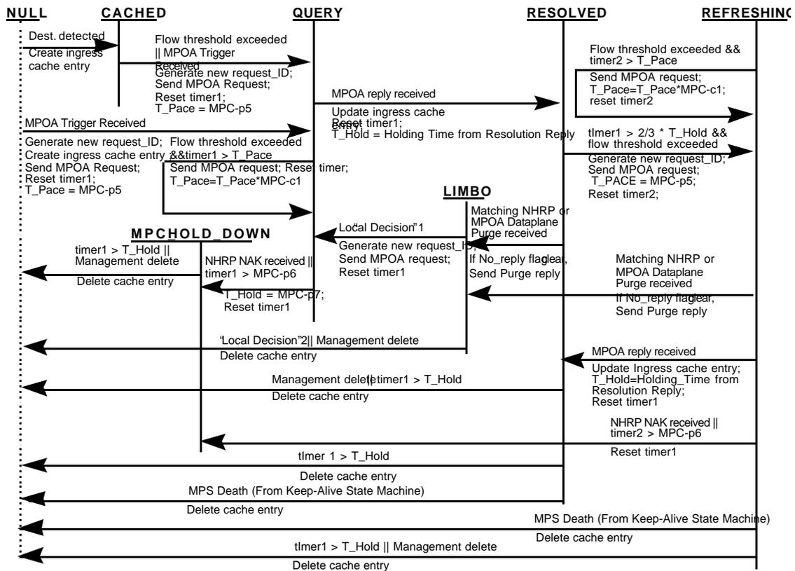
Figure 23 Ingress MPC Control State Machine
