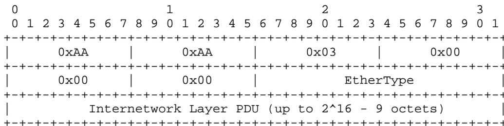
Figure 11 RFC 1483 LLC Encapsulation for Routed Protocols
