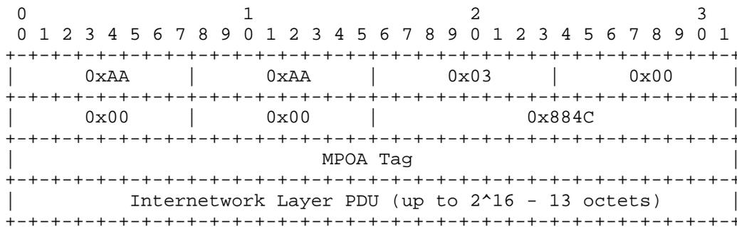
Figure 12 MPOA Tagged Encapsulation for Routed Protocols
