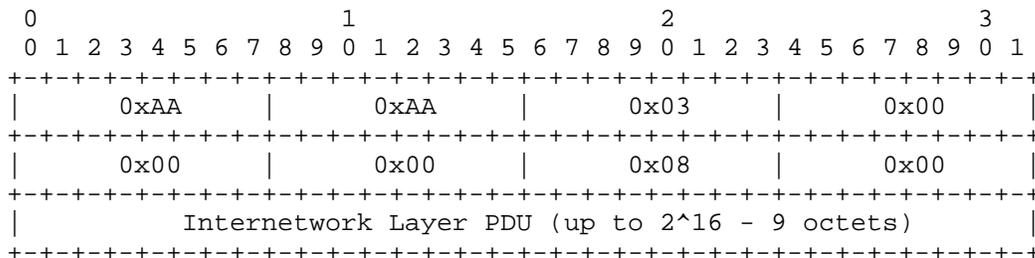
Figure 17 RFC 1483 LLC/SNAP Encapsulation for Routed IP PDUs
