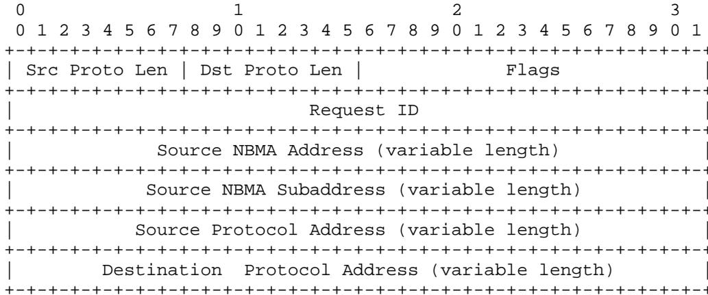
The Common Header specifies the sender's NBMA (ATM) and internetwork layer address and the receiver's internetwork layer address. Some exceptions exist in the context of certain MPOA control messages as described in the section for each message.
