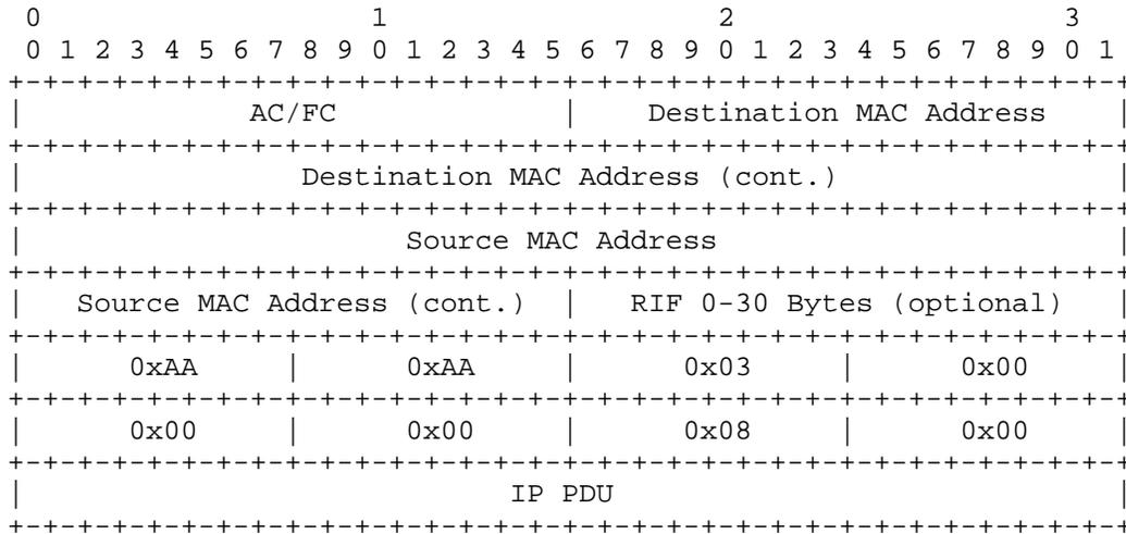
Figure 16 802.5 IP Encapsulation
