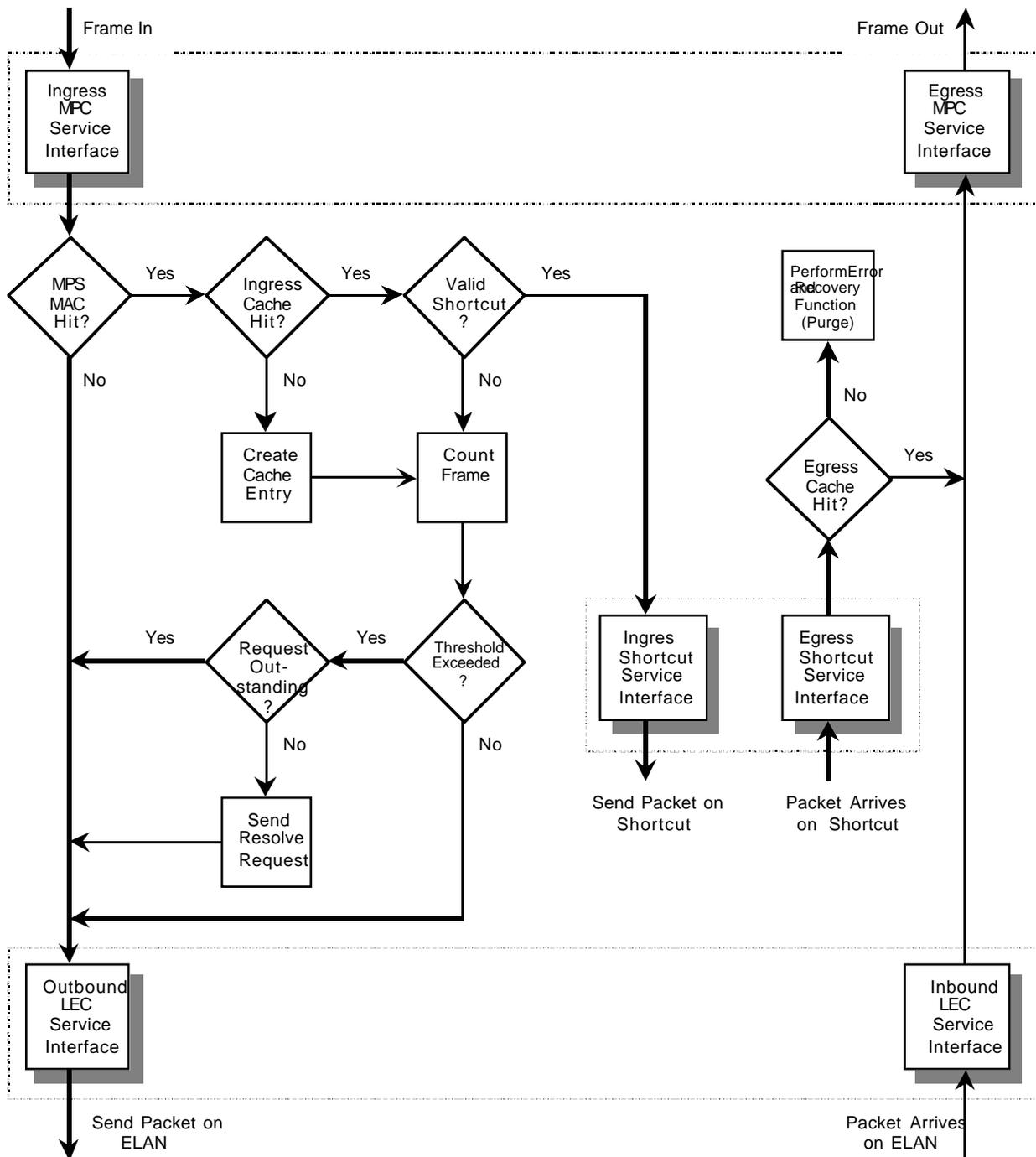
Figure 8 MPC Data Path Processing Logical Block Diagram
