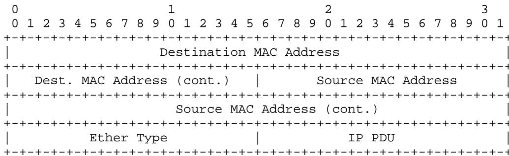
Figure 14 Ethernet IP Encapsulation
