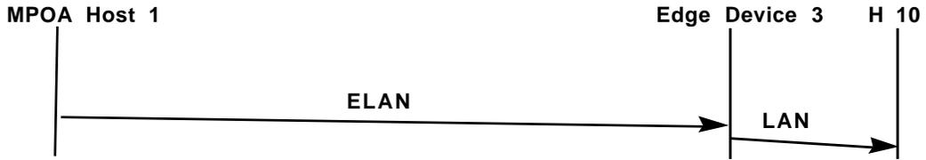
Figure 32 MPOA Host to LAN Host Data Flow
