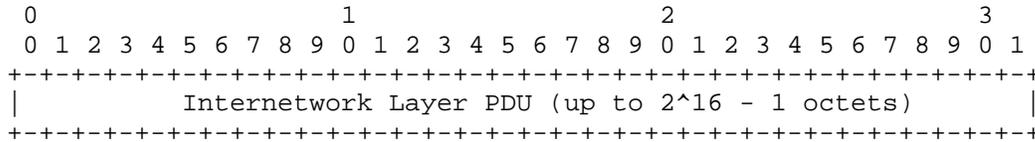
Figure 18 RFC 1483 “Null” Encapsulation for Routed IP PDUs
