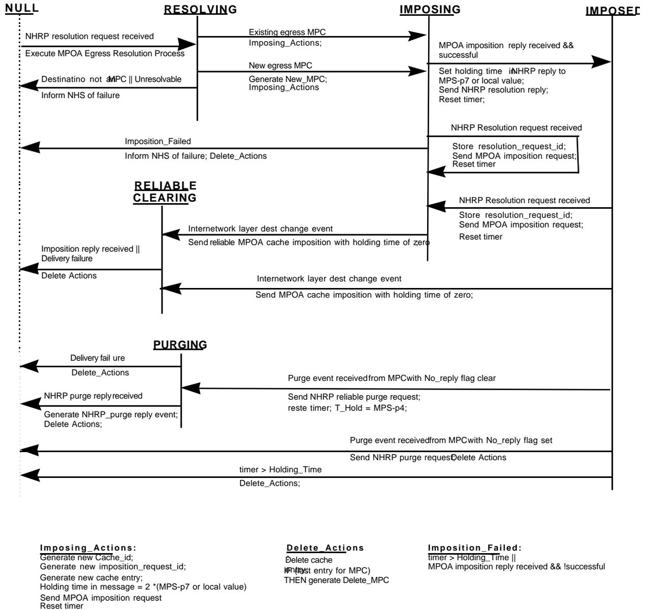
Figure 25 Egress MPS Control State Machine
