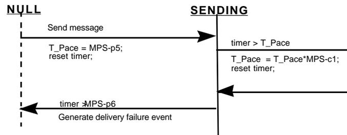
Figure 27 Reliable Delivery State Machines
