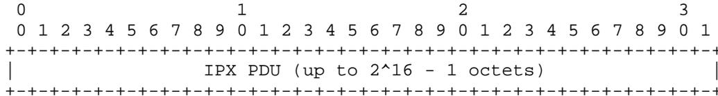
Figure 21 RFC 1483 "Null" Encapsulation for Routed IPX PDUs
