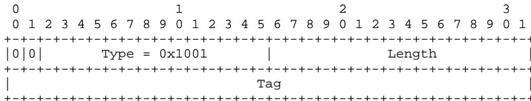
The tag is a 32 bit value chosen by the egress MPC.. A value of zero for the tag is not allowed
