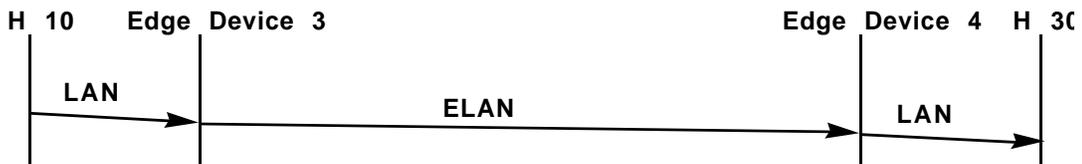
Figure 34 LAN Host to LAN Host Data Flow
