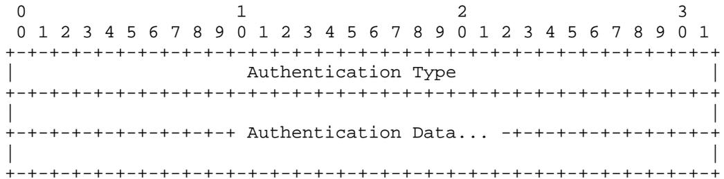
The Authentication Type field identifies the authentication method in use. Currently assigned values are:
