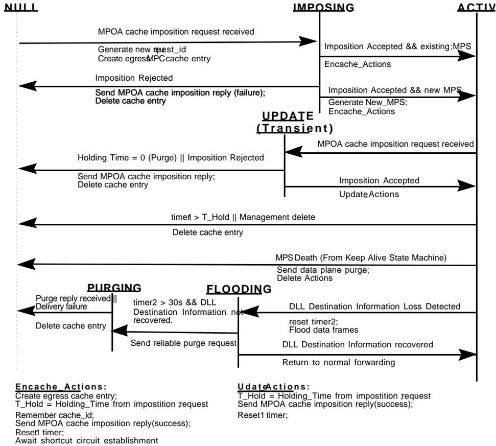
Figure 26 Egress MPC Control State Machine
