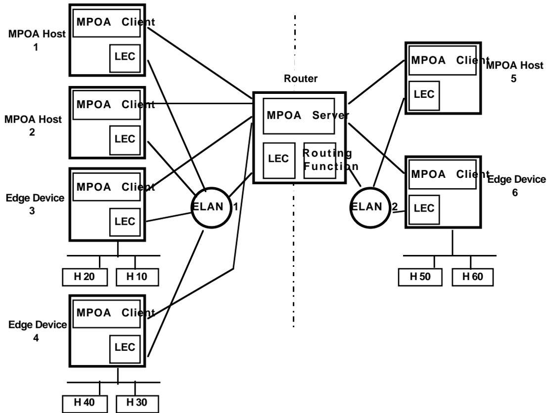
Figure 29 Example Network Configuration
