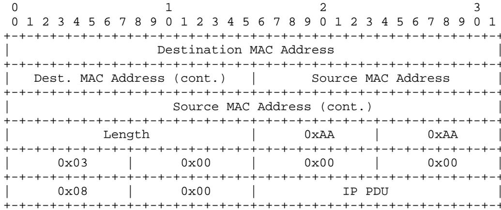
Figure 15 802.3 IP Encapsulation
