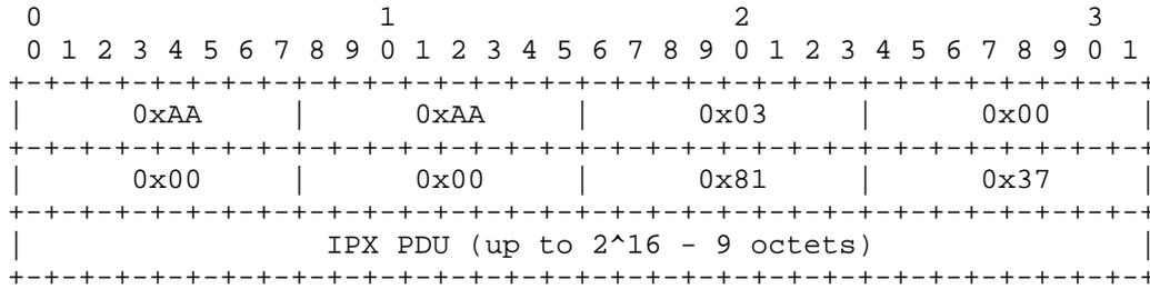
Figure 20 RFC 1483 LLC/SNAP Encapsulation for Routed IPX PDUs
