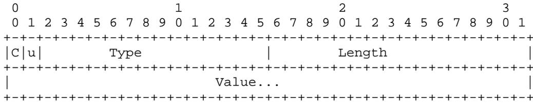
C "Compulsory." If clear, and the NHS does not recognize the type code, the extension may safely be ignored. If set, and the NHS does not recognize the type code, the NHRP "request" is considered to be in error. (See below for details.)
