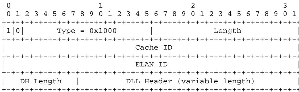
Cache ID specifies the egress MPS's ID for an egress cache entry. A value of zero for the cache ID is not allowed.
