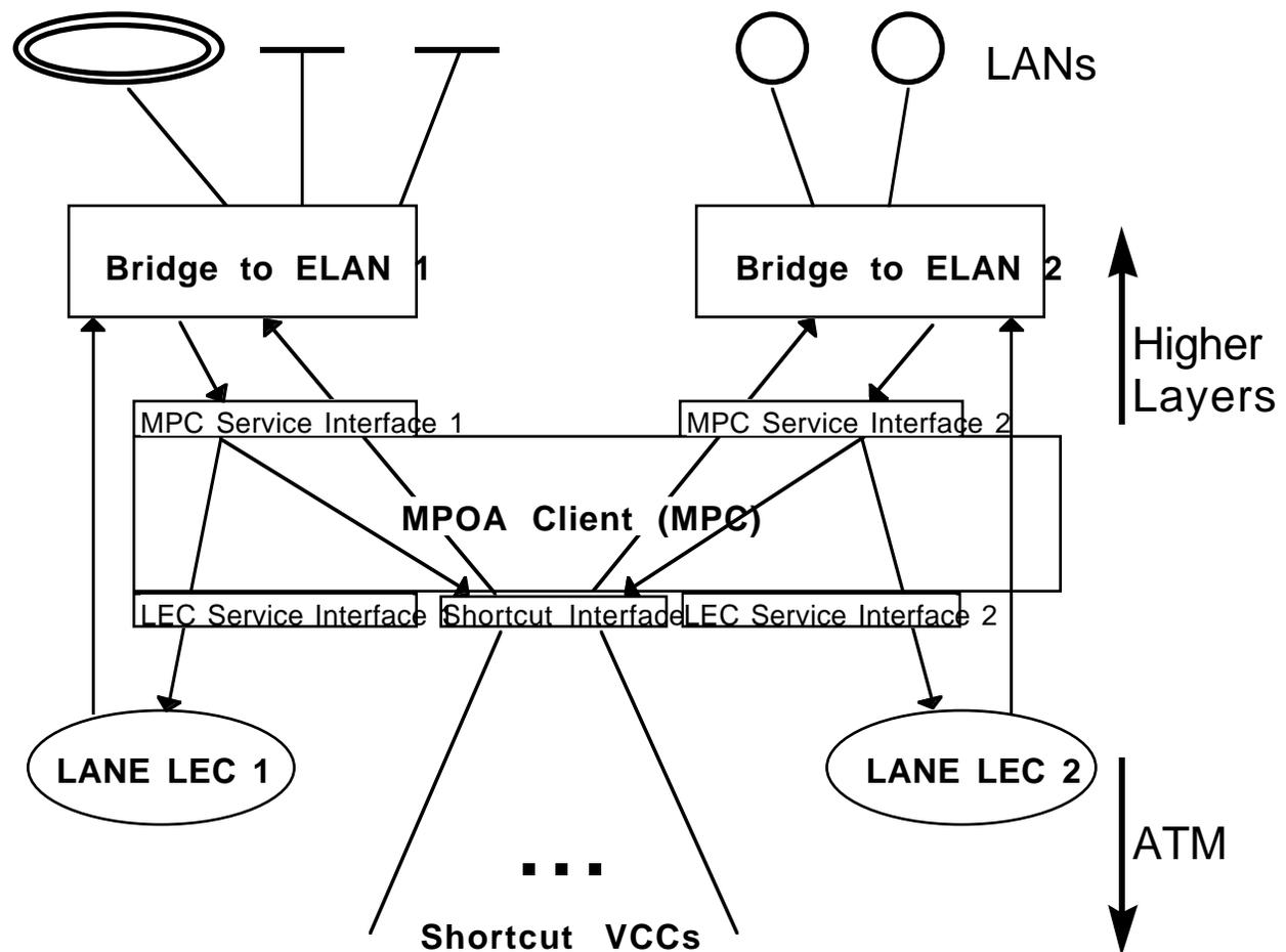
Figure 7 MPOA Edge Device MPC Example
