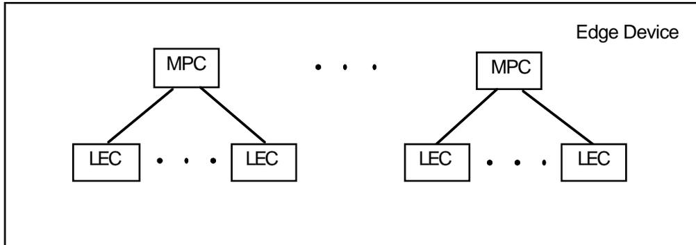
Figure 2 Relationship Between LECs, MPCs, and Edge Devices
