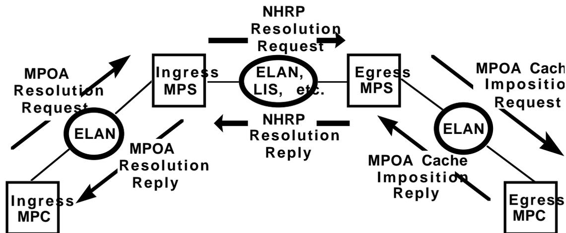
Figure 10 MPOA Resolution Process
