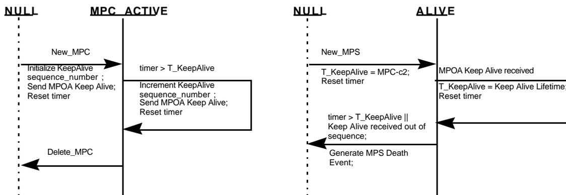
Figure 28 Egress MPC and MPS Keep-Alive State Machines
