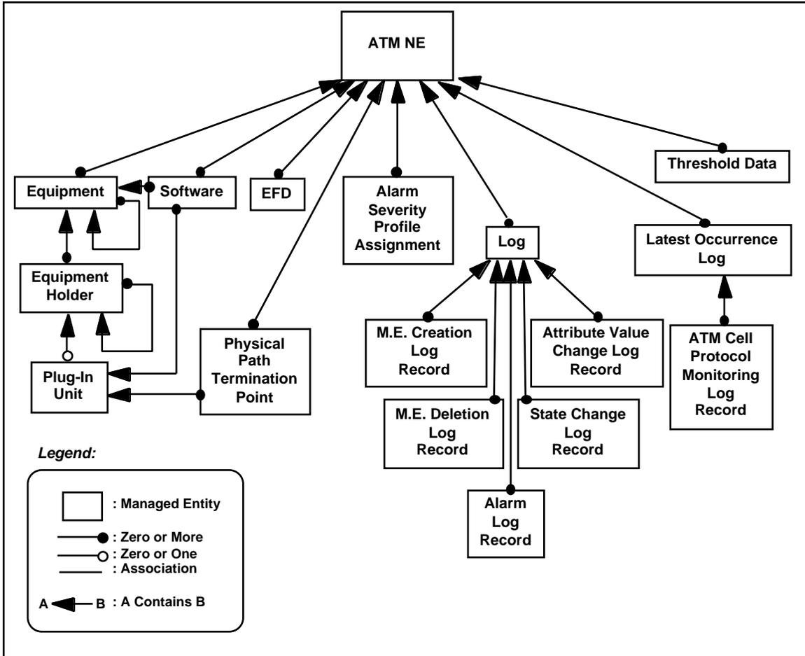
Figure 3-3 Managed Entity Relationship Diagram (3 of 3)
