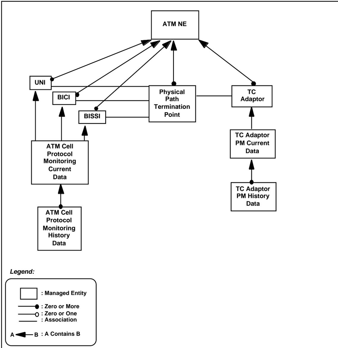
Figure 3-2 Managed Entity Relationship Diagram (2 of 3)
