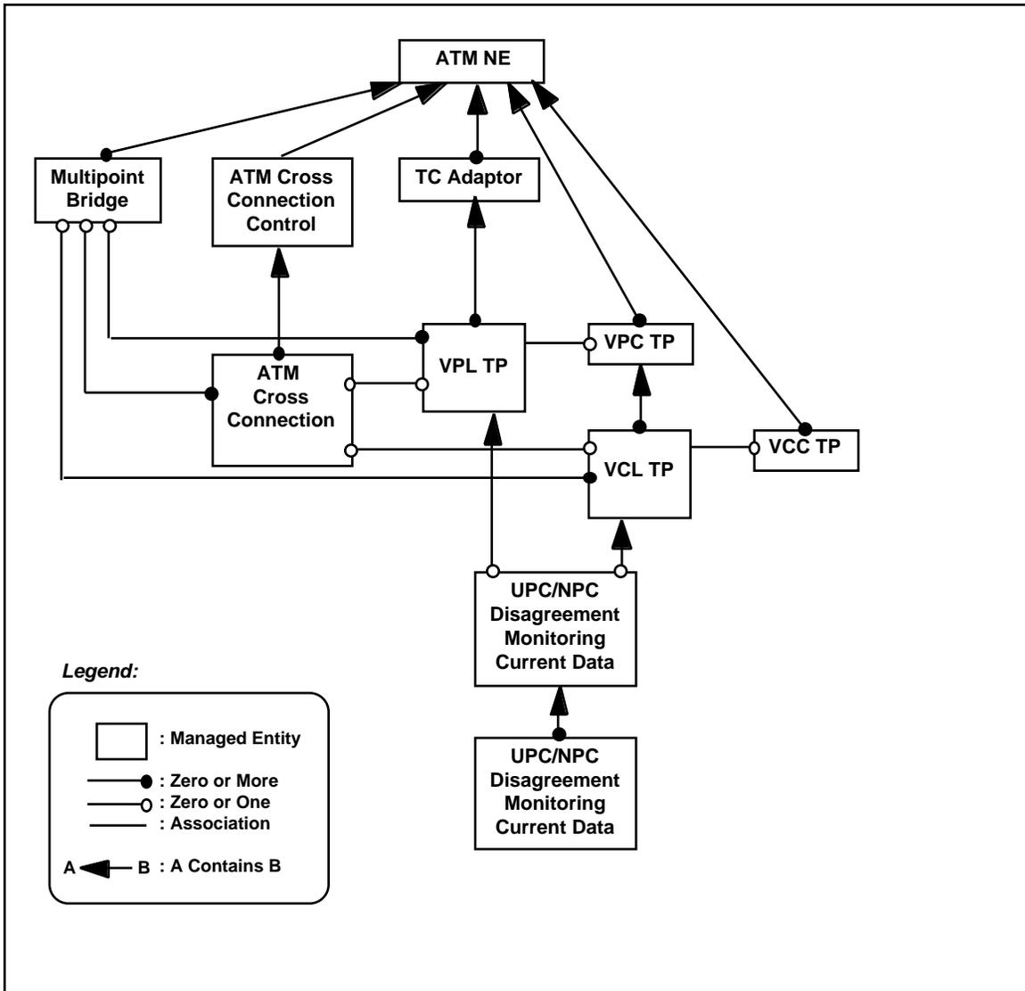
**Figure 3-1** Managed Entity Relationship Diagram (1 of 3)
