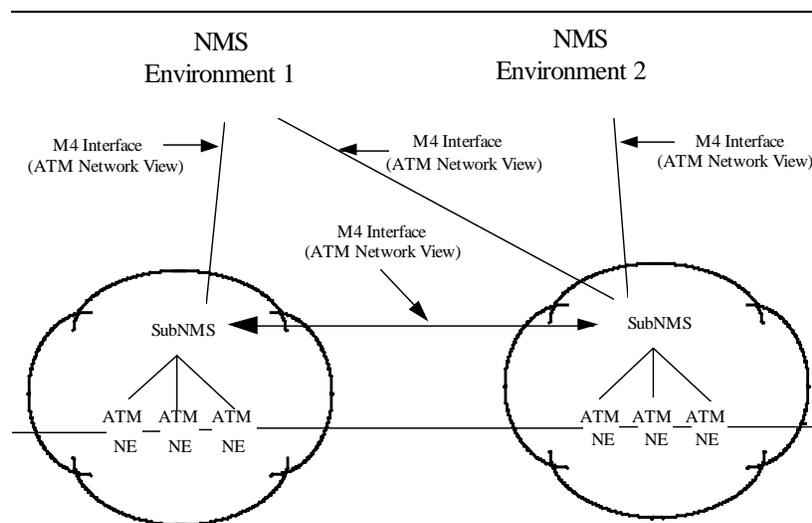
**Figure 3-4-2: Example of Multi-Manager Management Physical Configuration**
