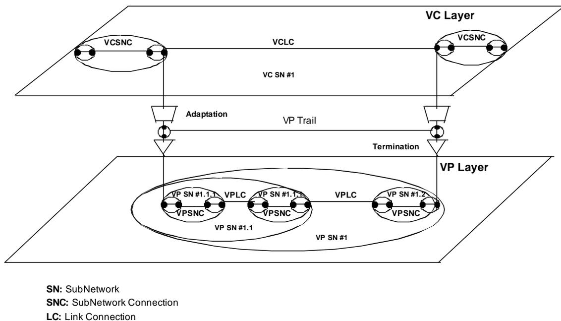
**Figure 2-1: Functional Representation of a Subnetwork Connection**
