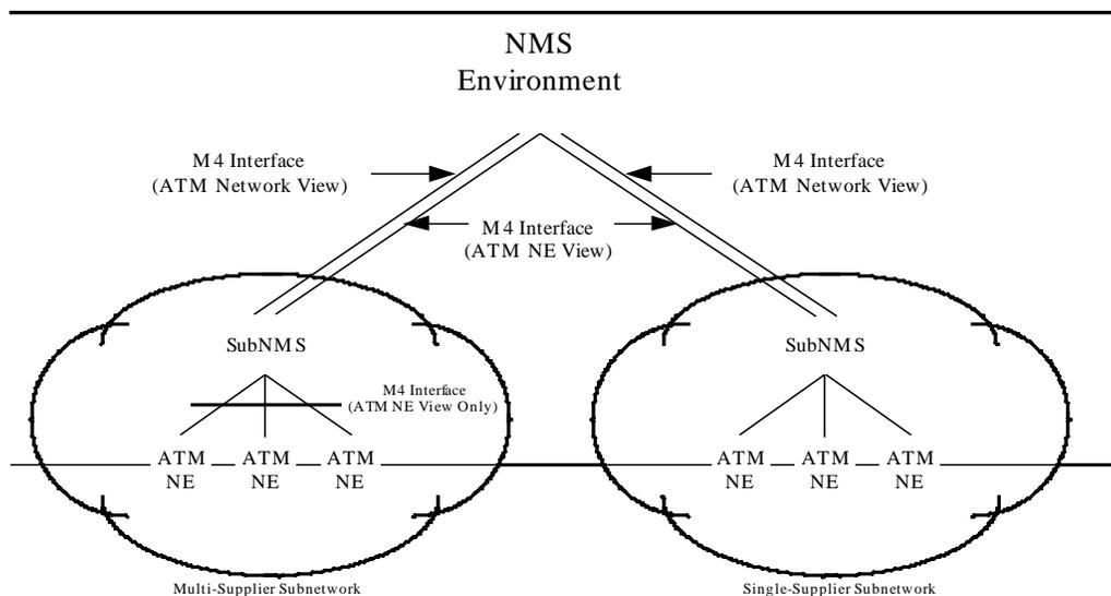
**Figure 3-3-1: Example of NE+Network-Level Management Physical Configuration**
