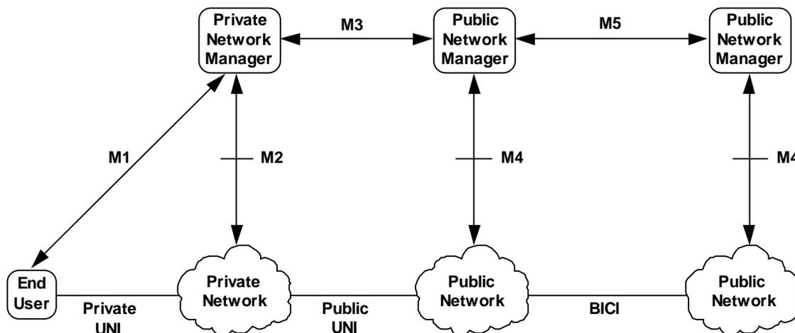
**Figure 1-1 The ATM Forum Management Interface Reference Architecture**
