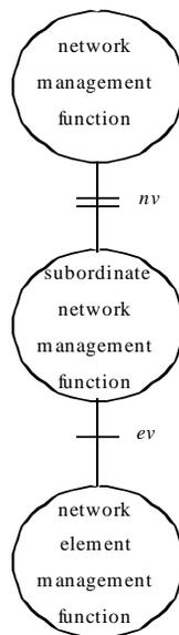
**Figure 3-1: M4 Network-View Logical Architecture**
