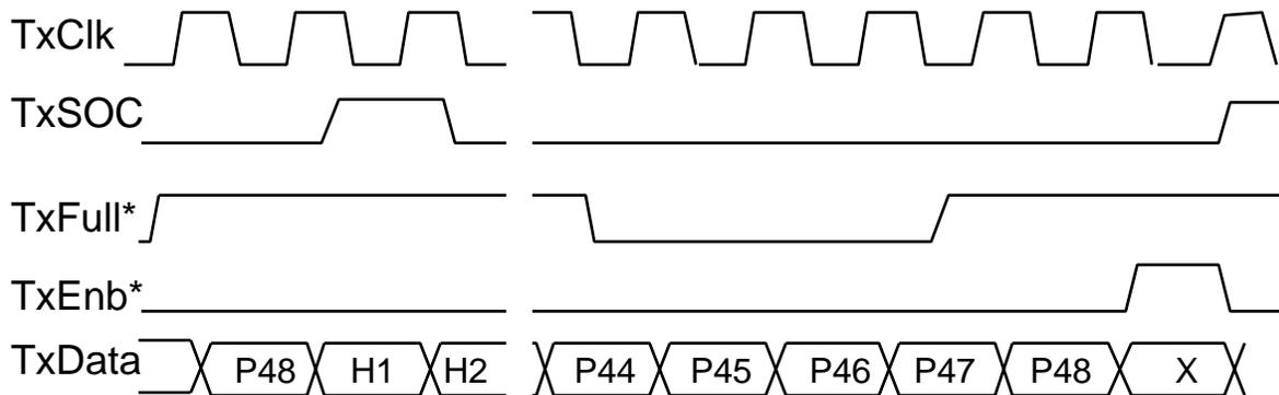
**Figure 4. Transmit Timing for Cell-Level Handshake**
