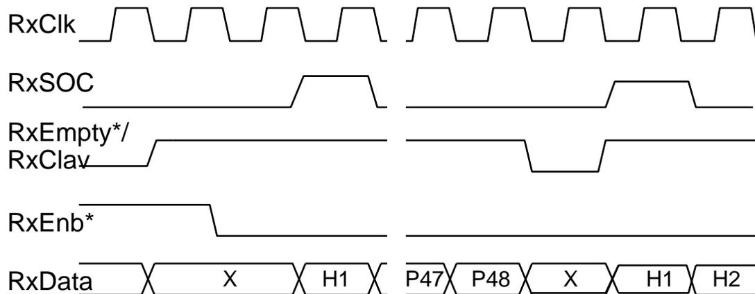
**Figure 7. RxEmpty\*/RxClav Timing**
