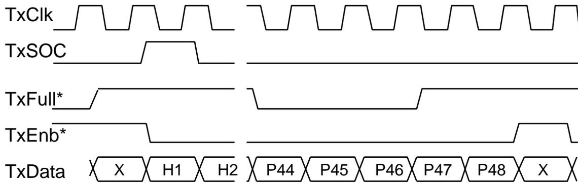
**Figure 3. Transmit Timing for Octet-Level Handshake**
