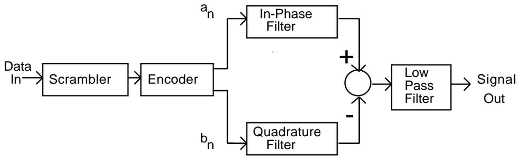
**FIGURE 2-2 BLOCK DIAGRAM OF DIGITAL 16-CAP TRANSMITTER FUNCTIONALITY**
