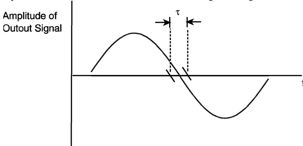
FIGURE 2-1 ILLUSTRATION OF TRANSMITTER JITTER
