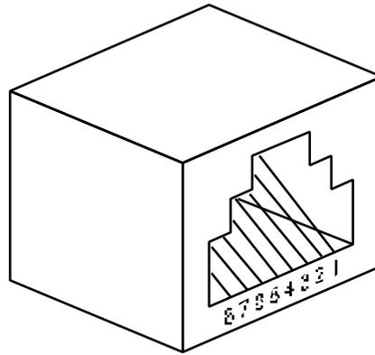
**FIGURE 2-10 EXAMPLE OF A UTP-MIC JACK**
