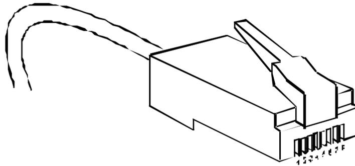
FIGURE 2-9 EXAMPLE OF A UTP-MIC MODULAR PLUG
