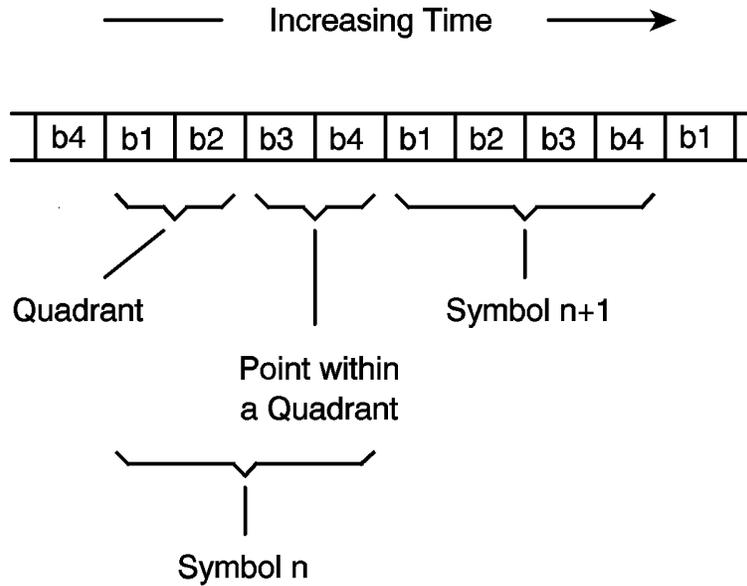
**FIGURE 2-3 BIT-TO-SYMBOL MAPPING FOR 16-CAP**
