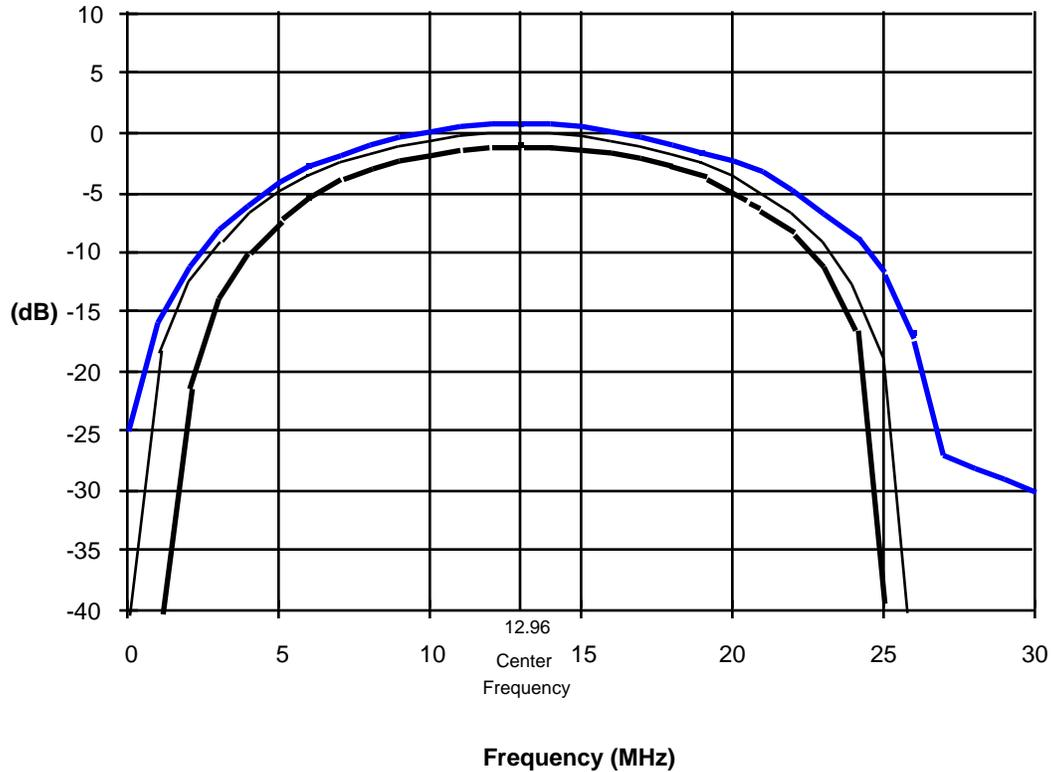
**FIGURE 2-8 TEMPLATE FOR THE POWER SPECTRUM OF THE SIGNAL AT THE OUTPUT OF THE TRANSMITTER**
