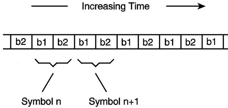
**FIGURE 2-5 BIT-TO-SYMBOL MAPPING FOR 4-CAP**
