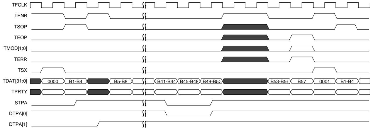
When DTPA transitions low and it has been sampled, the Link Layer device can write no more than a predefined number of bytes to the selected FIFO. In this example, the predefined value is two double-words or eight bytes. If the Link Layer writes more than that predefined number of words and DTPA remains deasserted throughout, the PHY layer device should indicate an error condition and ignore additional writes until it asserts DTPA again.
