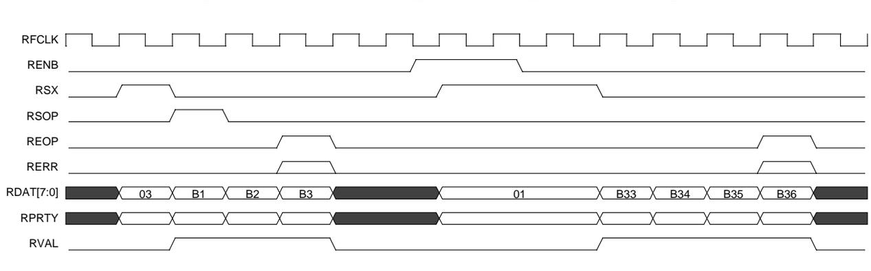
Figure 7.3 shows an example of data transfer from a single-port PHY device, without the use of the RSX signal and in-band addressing, which are optional for single-port applications. Just before reaching end-of-packet, the PHY device happens to pause for two cycles (for internal reasons).
