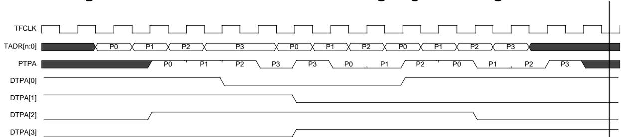
Figure 6.3 shows an example of data transfer to a single-port PHY device without the use of in-band addressing, which is optional for single-port applications. During packet transfer, the Link Layer device pauses for its own internal reasons. As in Figure 6.1, the PHY device indicates its FIFO status by means of DTPA.
