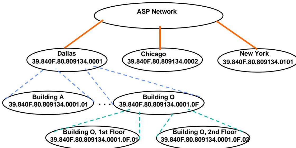
Figure 4 Hierarchical Network Structure without Address Aggregation
