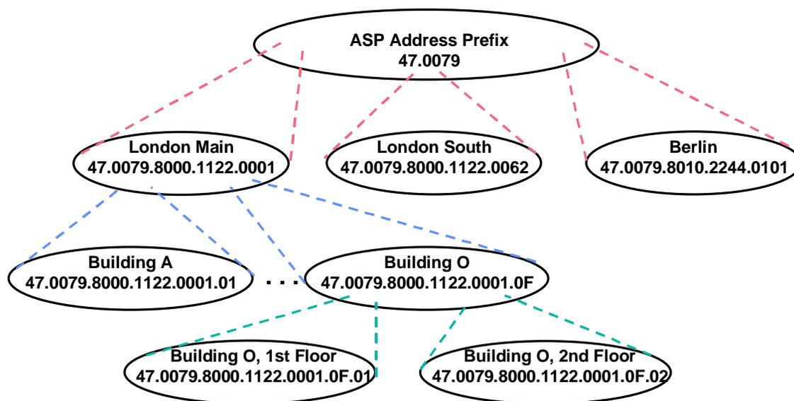
Figure 5 Hierarchical Network Structure with Address Aggregation
