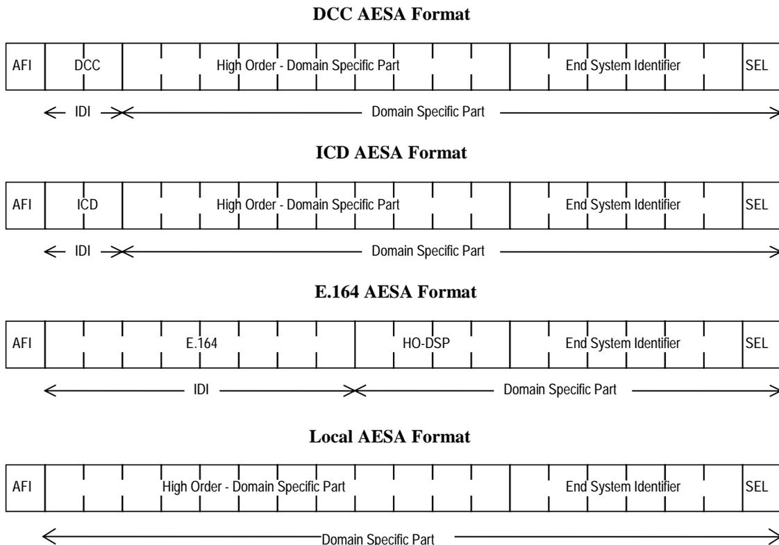
**Figure 1 ATM Forum Defined ATM End System Address Formats**
