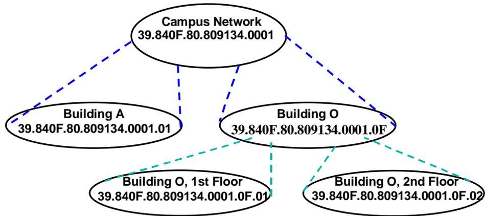
Figure 3 Campus Network with Address Aggregation
