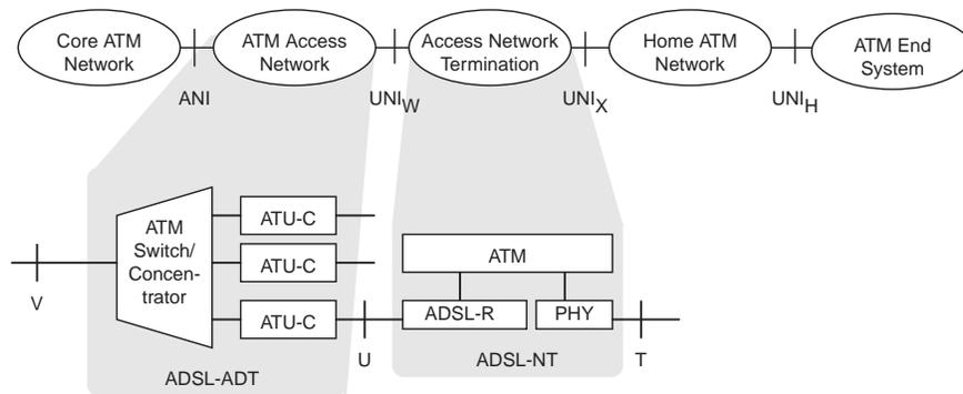
**Figure 3-7 Mapping of ADSL (Active NT) Functional Model on the RBB Reference Architecture**
