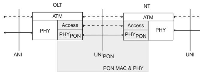
**Figure 3-4 ATM Transport Protocol Model**
