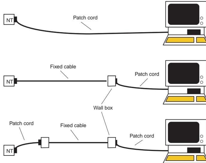
**Figure 4-3 Patching Configuration**
