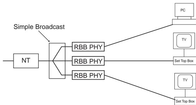
**Figure A-2 VDSL interface to multiple ATM interfaces using simple broadcast**
