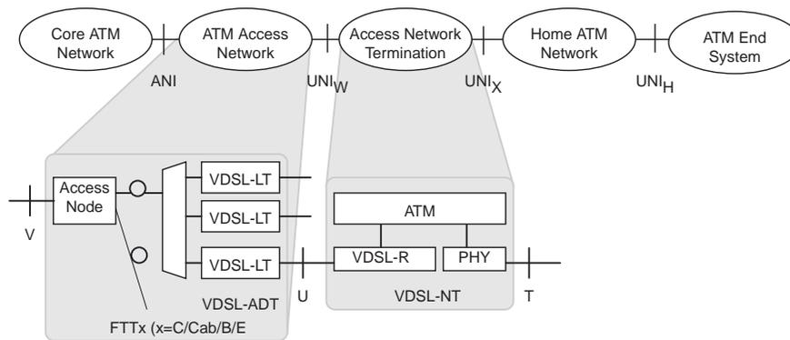
**Figure 3-8 Mapping of VDSL (Active NT case) Functional Model on the RBB Reference Architecture**
