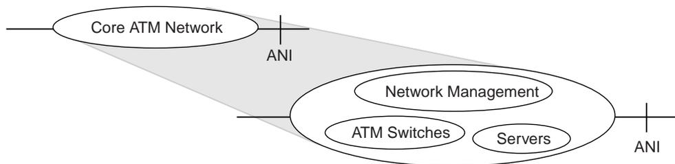
Figure 1-2 Functional Decomposition of the Core ATM Network
