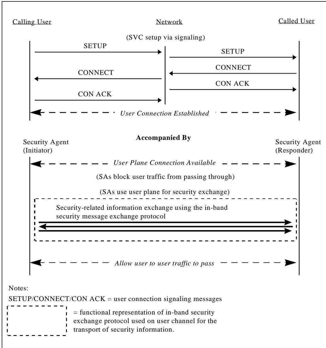
**Figure 24: Point-to-Point Security Exchange Using the Hosts' User Plane for SVCs.**
