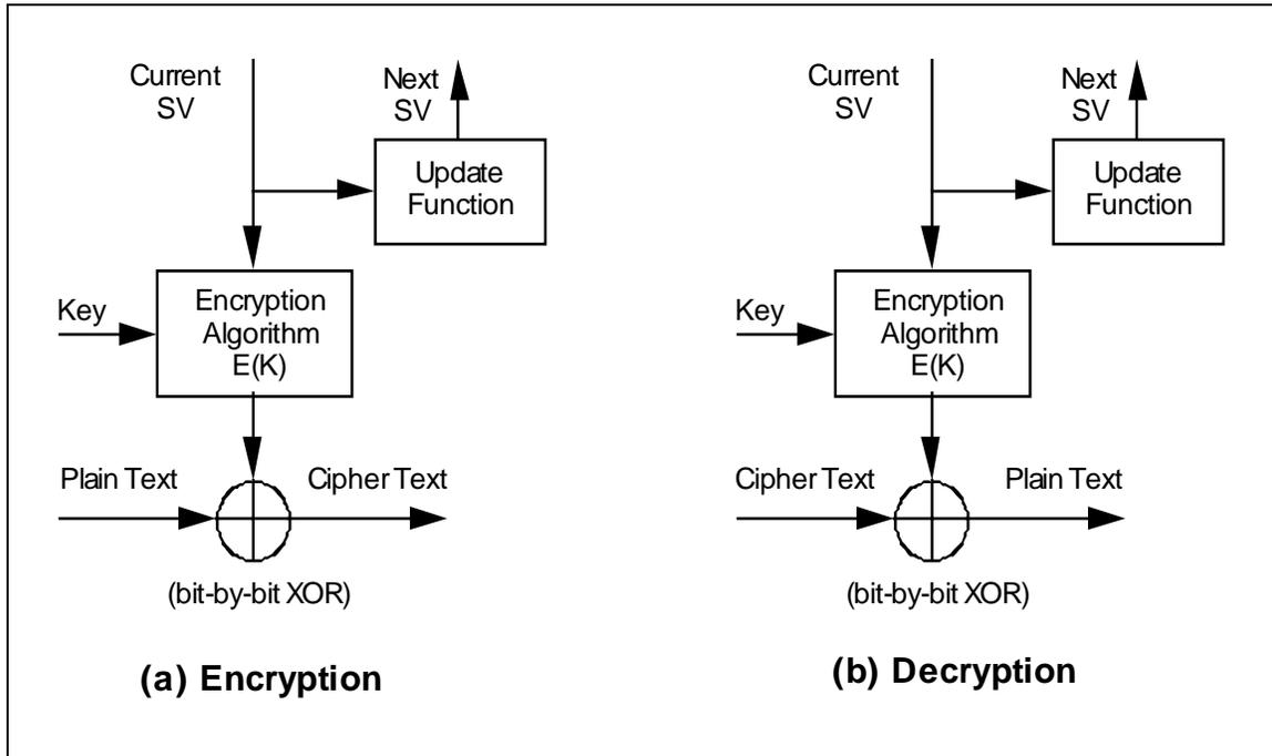
Figure 40: Counter Mode Block Diagram.
