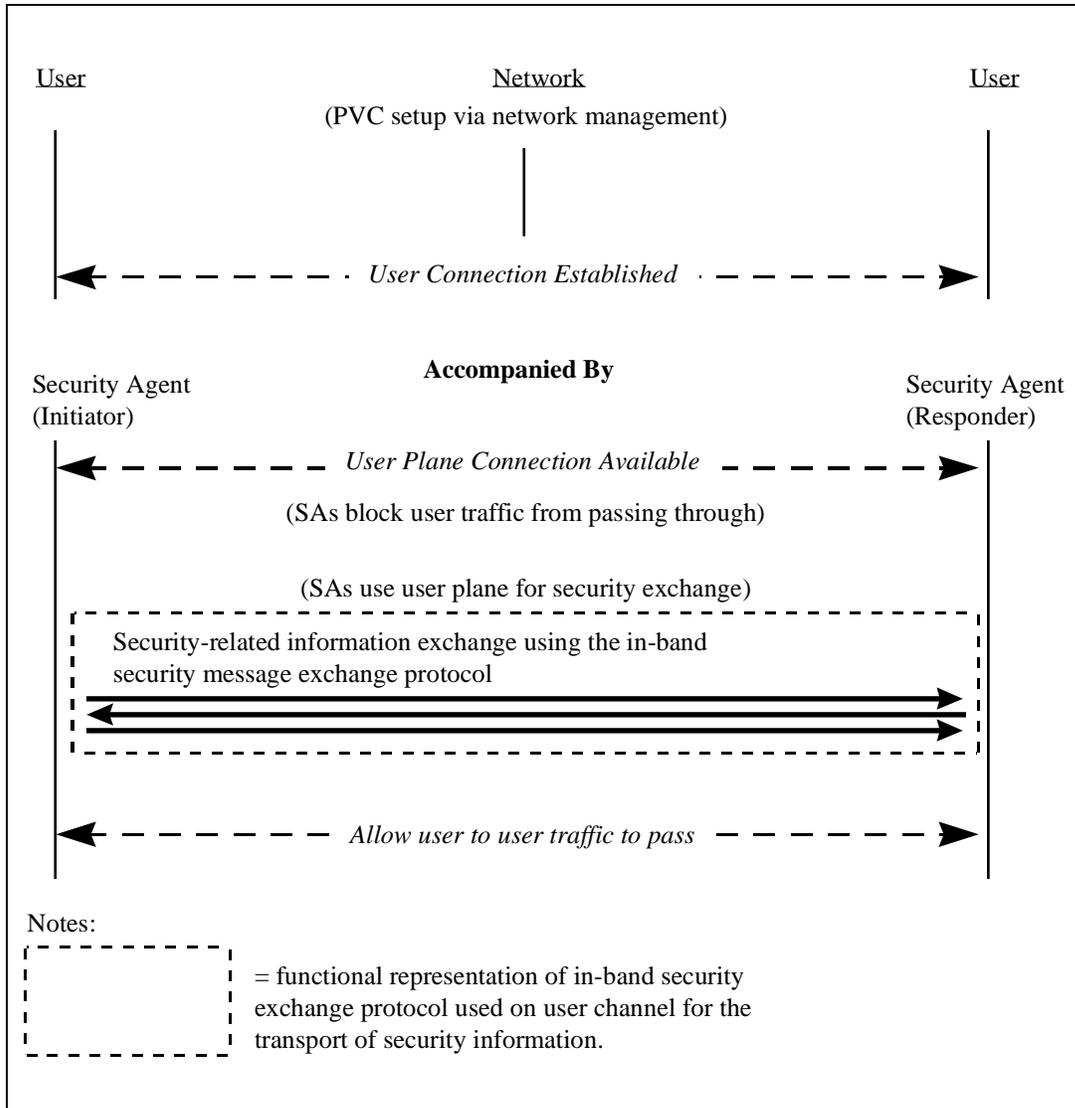
**Figure 25: Point-to-Point Security Exchange using the Hosts' User Plane for PVCs.**
