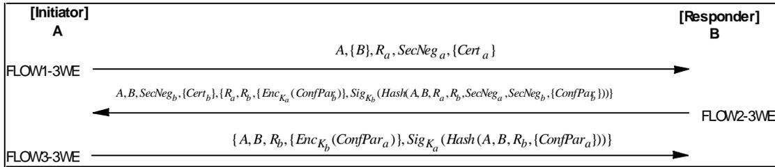
**Figure 20: Three-Way Security Message Exchange Protocol.**
