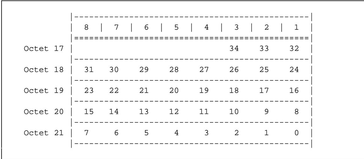
Figure 48: Jump Number Position within SKC OAM Cell.
