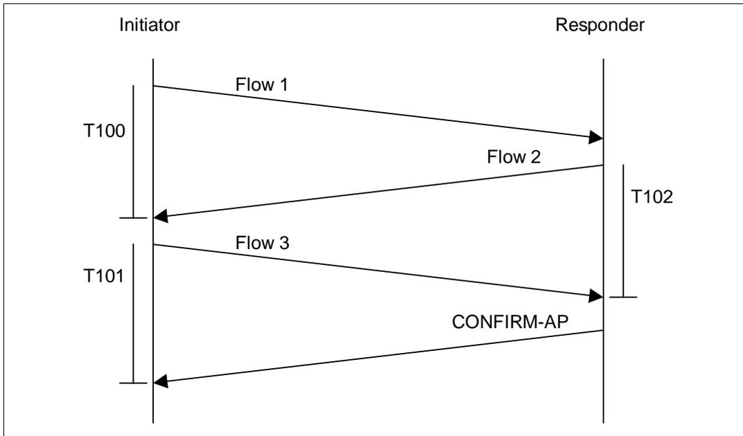
**Figure 36: Basic Message Exchange Sequence.**
