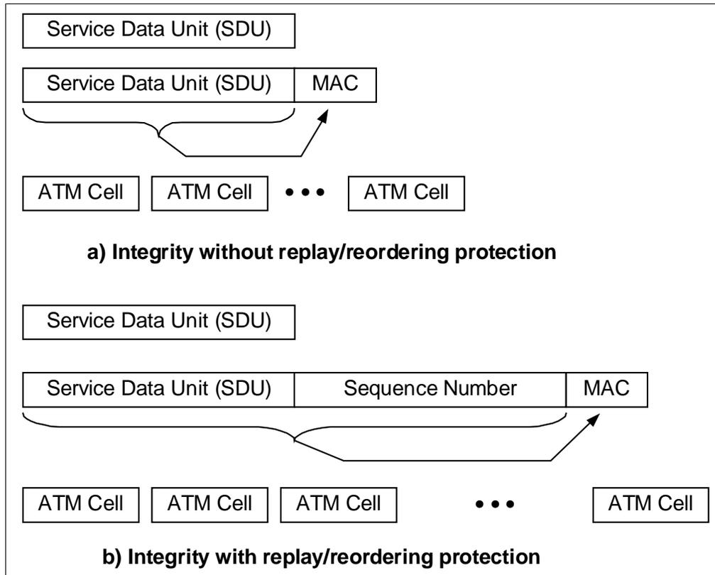
**Figure 16: AAL-SDU Level Data Integrity.**
