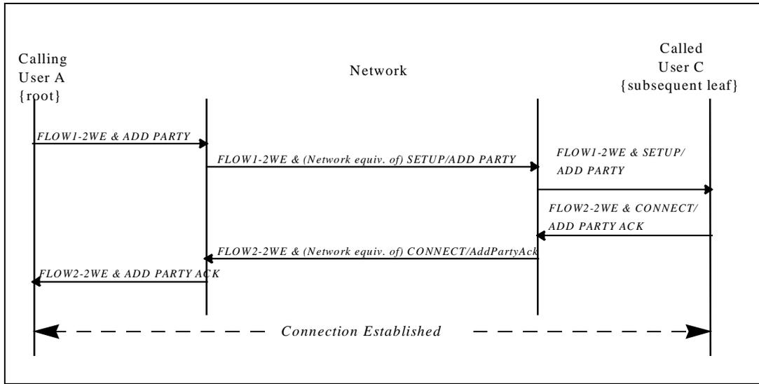
**Figure 23: Point to Multipoint Signaling Support for Two-Way Security Message Exchange for Subsequent Leaf Setup.**
