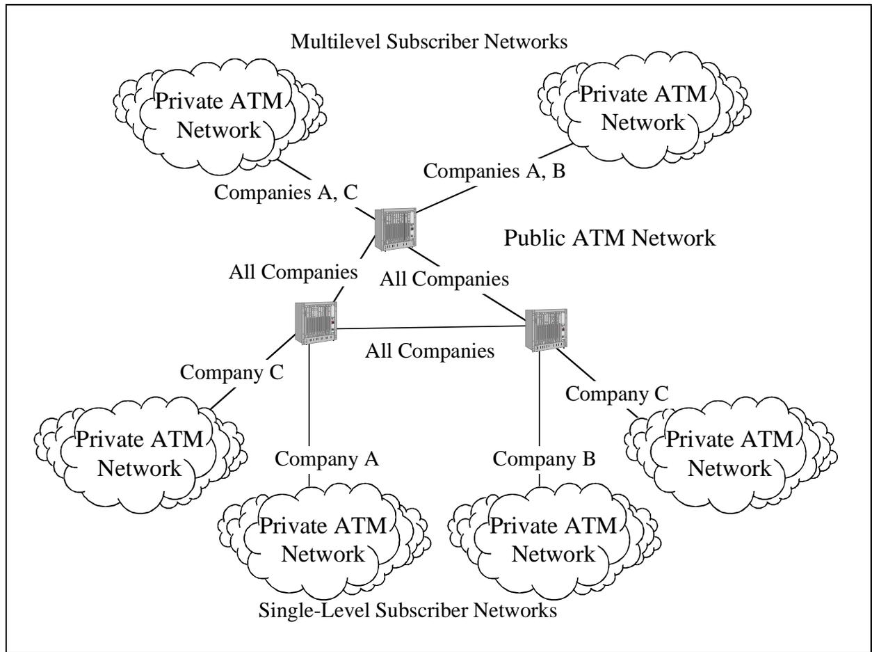
**Figure 53: Access Control Scenario for Public Switches.**
