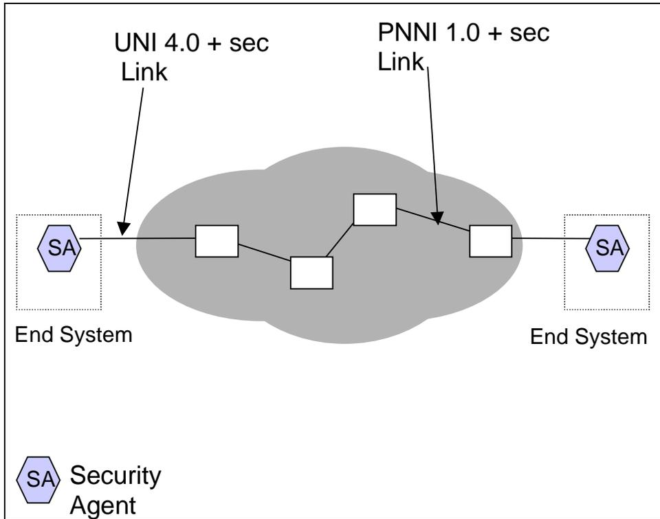
**Figure 7: Entire Network Supports Signaling-Based SME.**
