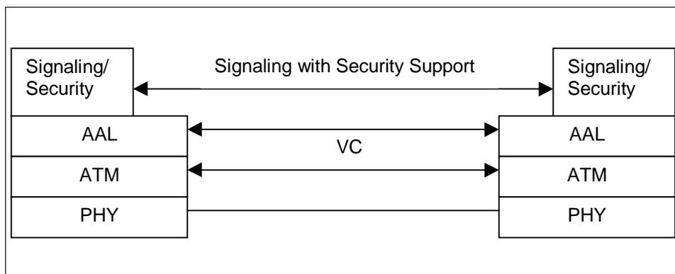
**Figure 17: Access Control Layer Reference Model for Signaling-Based Messaging.**
