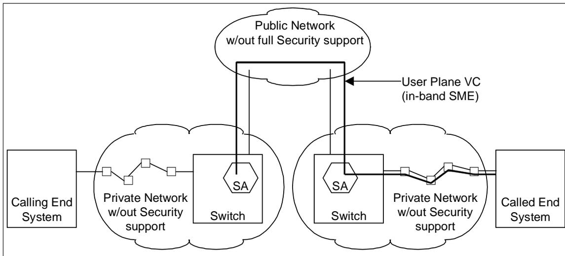
**Figure 9: Using the In-Band SME Protocol in Networks that do not support Signaling-Based SME.**
