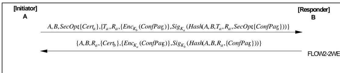
**Figure 21: Two-Way Security Message Exchange Protocol.**
