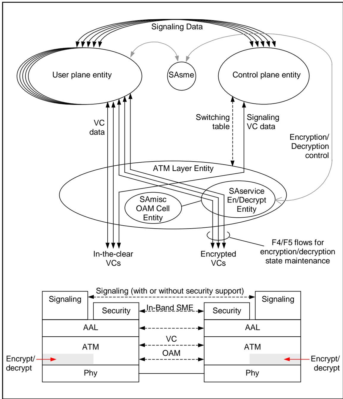
Figure 13: Object and Layer Reference Models for Confidentiality with In-Band SME.
