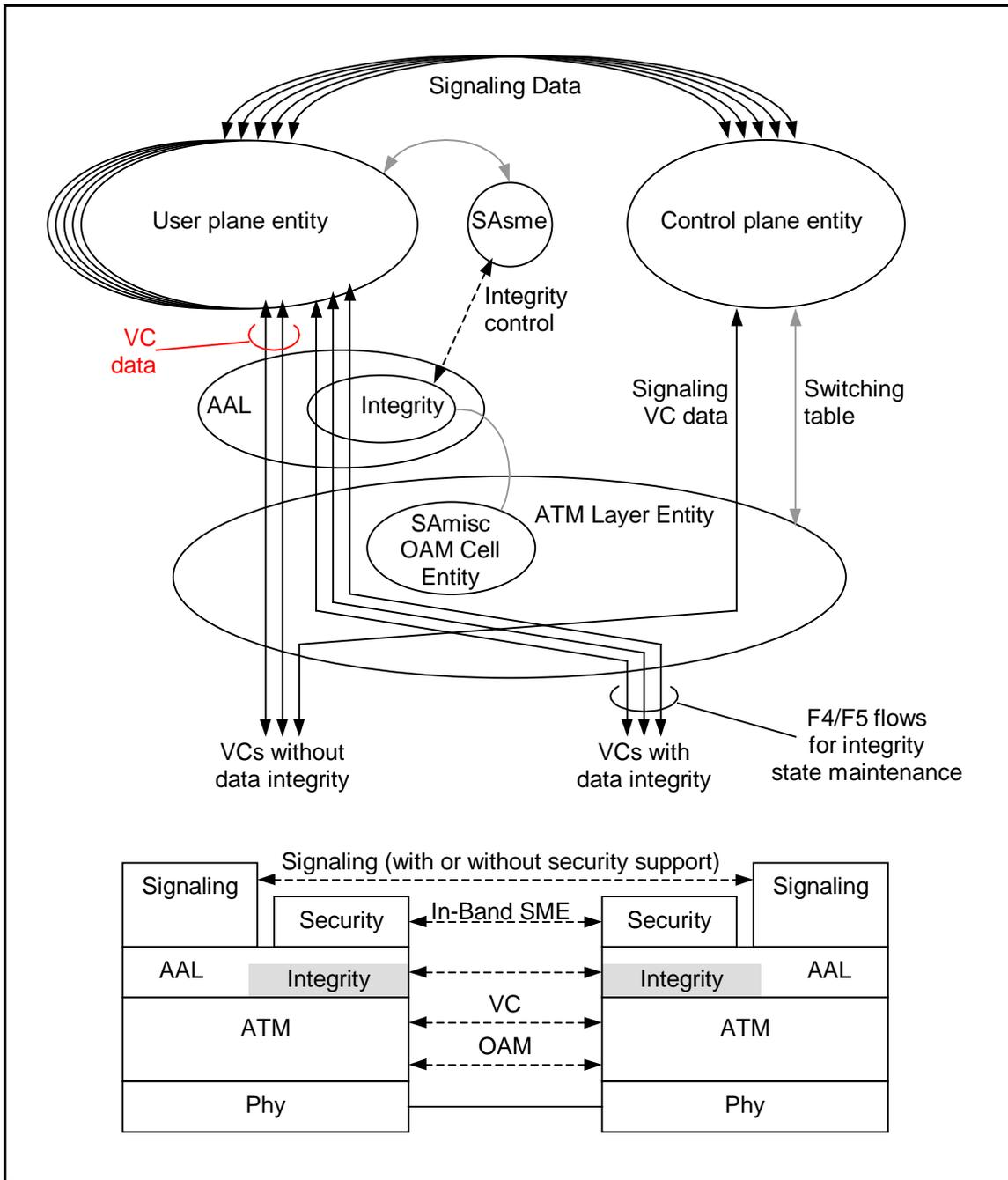
Figure 15: Object and Layer Reference Models for Data Integrity with In-Band SME.
