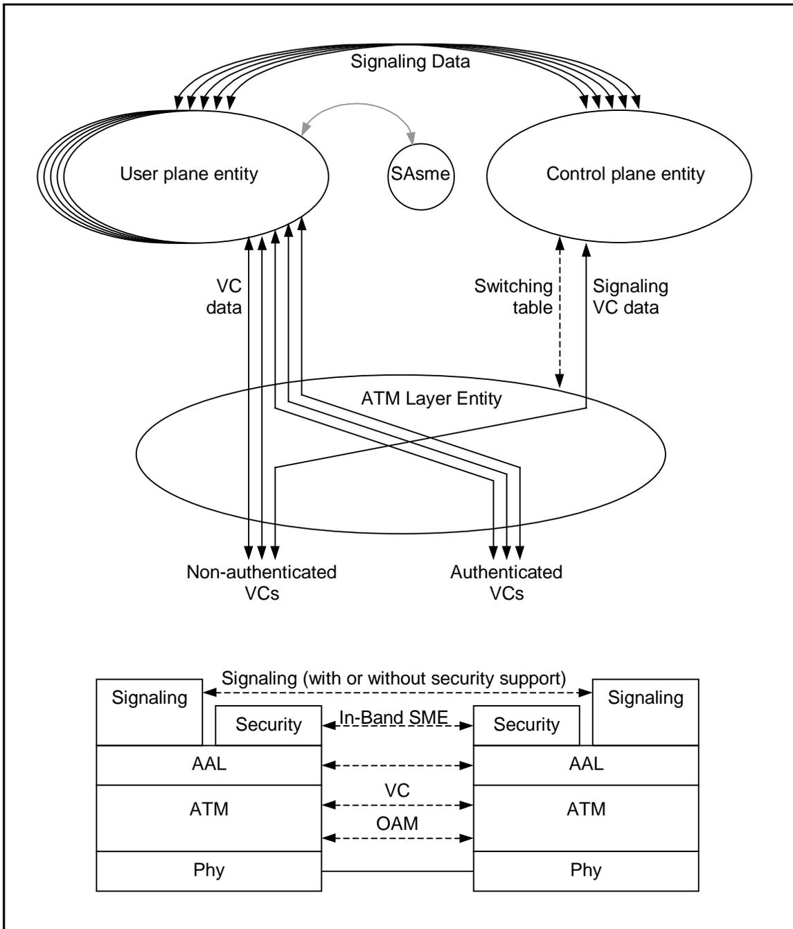
**Figure 11: Object and Layer Reference Models for Authentication with In-Band SME.**
