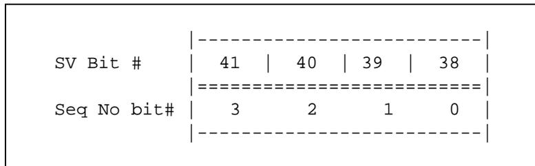
**Figure 45: Sequence Number Bit Format.**
