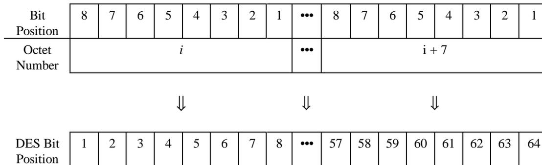
**Figure 39: Symmetric Encryption Algorithm Key Bit Ordering.**
