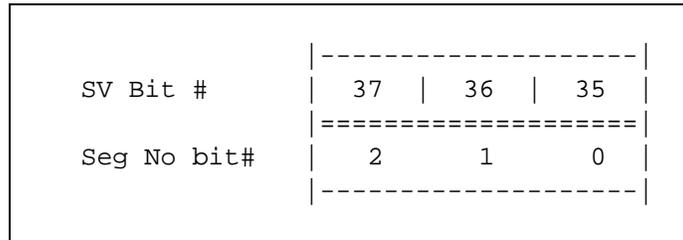
**Figure 46: Segment Number Bit Format.**
