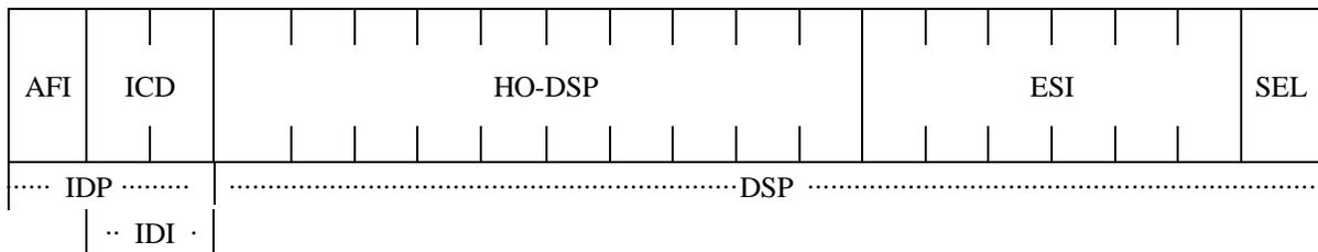
**Figure 3-1b ICD ATM Format**
