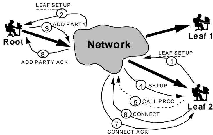
*Figure B-5. Leaf join to active Root LIJ call, where Root connects Leaf*
