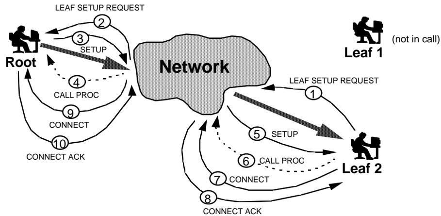
Figure B-3. Leaf join to inactive call, where Root connects Leaf
