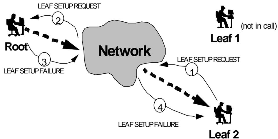
Figure B-4. Unsuccessful Leaf join to an inactive call.
