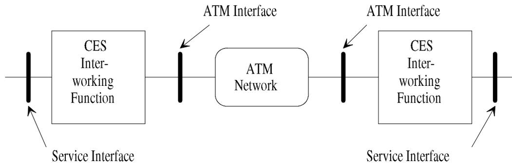
**Figure 5-1: Reference Network Configuration**
