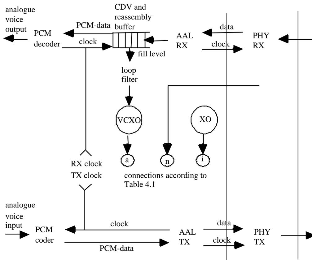
Figure 4-3 Timing relationships in the B-TE
