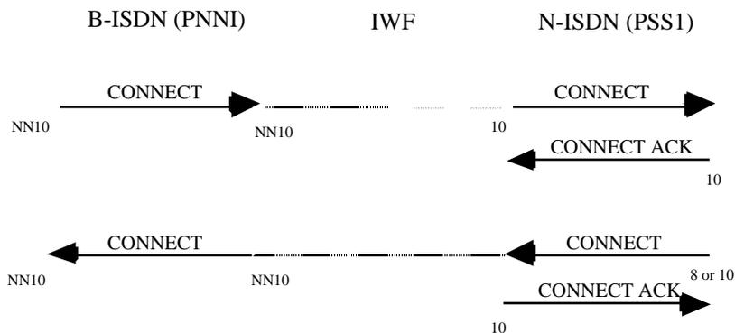
**Figure 3-7 Mapping of connection establishment messages in private N-ISDN/private B-ISDN**
