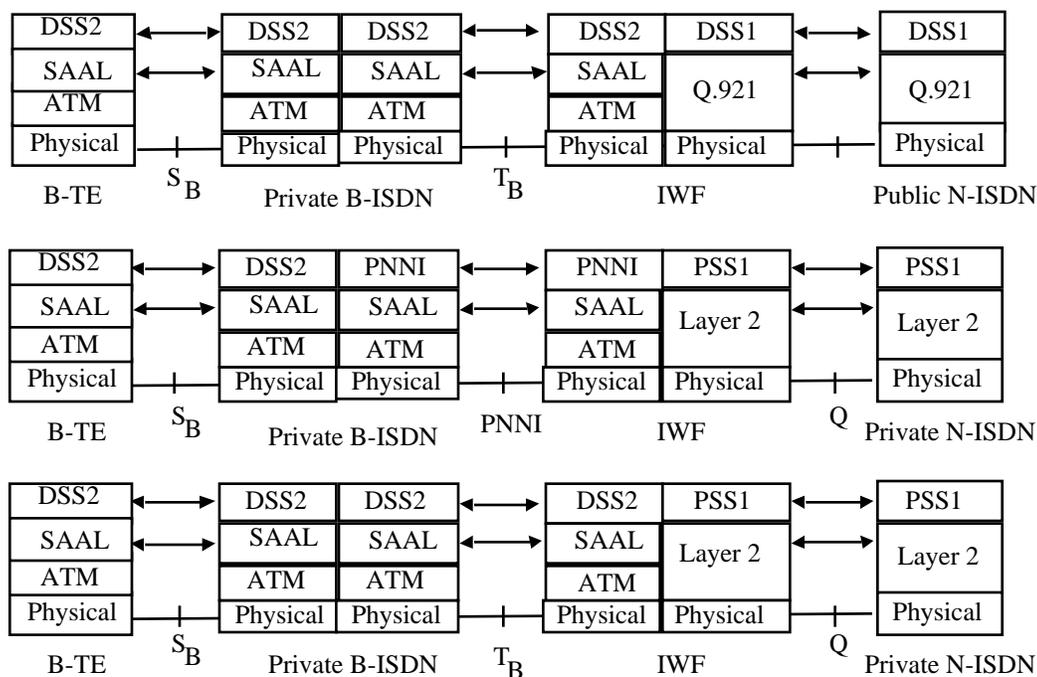
**Figure 3-4 Signalling (C-plane)**
