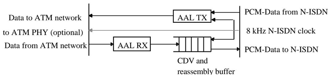
Figure 4-2 Basic structure of the IWF
