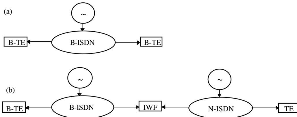
Figure 4-1 Network Based Timing Distribution Mechanisms
