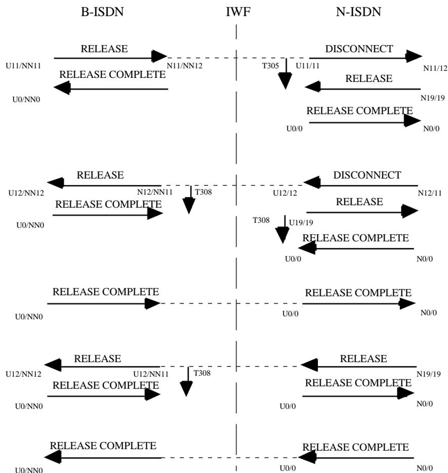
**Figure 3-5 Mapping of call clearing messages**
