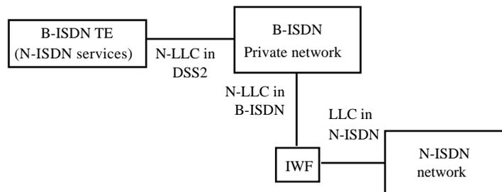
**Annex E/Q.2931 Mapping functions to support 64 kbit/s based circuit-mode ISDN services in B-ISDN and interworking between N-ISDN and B-ISDN (DSS1/DSS2):** Since this specification is applicable at both the UNI and at the PNNI, "DSS1" shall be replaced by "N-ISDN", and "DSS2" shall be replaced by "B-ISDN" throughout Annex E. The modifications of UNI SIG 4.0 apply.
